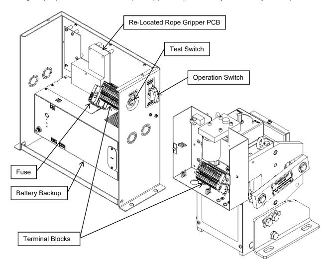
Figure 30 - Emergency Power Unit Key Components
