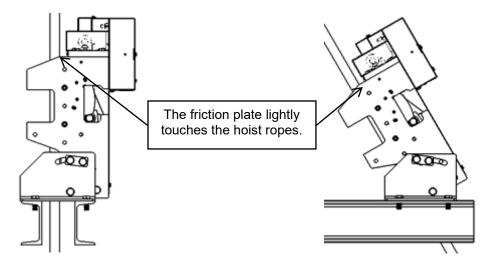
Figure 10 - Stationary Shoe Contact
