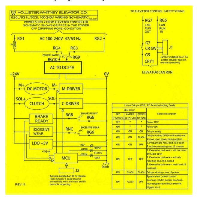
Figure 29 – Wiring Schematic
