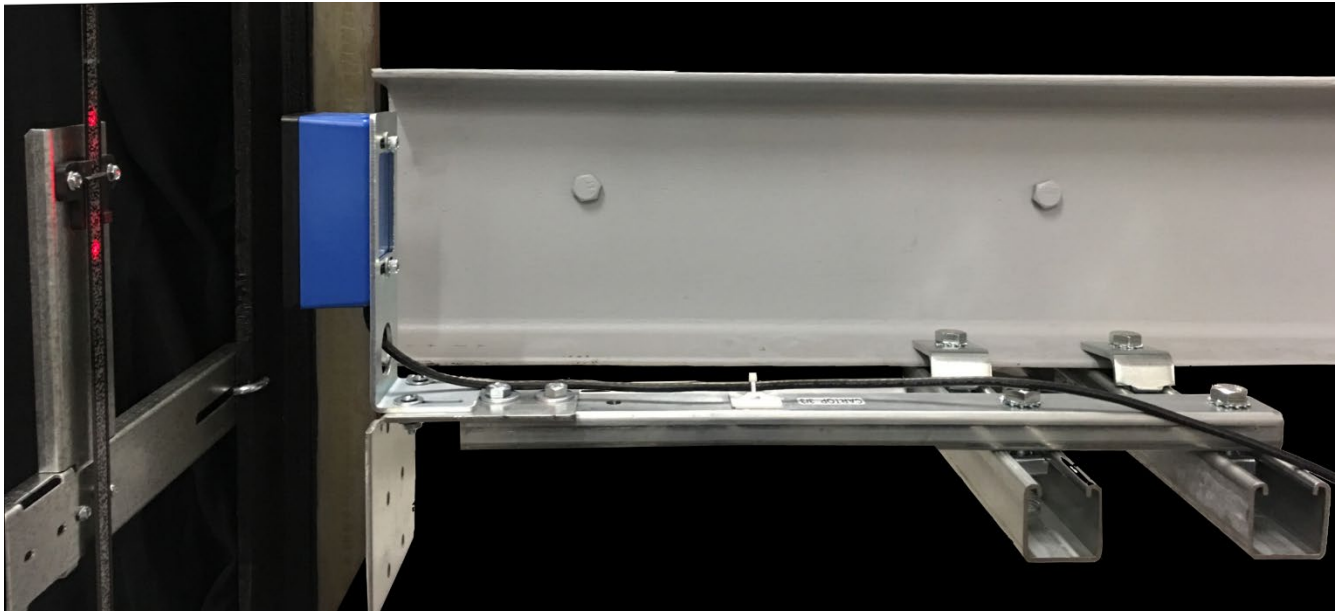
Figure E1.7: CEDES APS Camera Mounting Bracket
