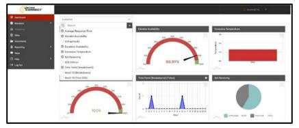
The graphical dashboard shows an at-a-glance view of key performance indicators such as equipment availability, equipment out of service, site performance, alarm trappings and much more. Customize your own dashboard to suit your requirements using the simple drag and drop features.
