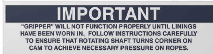
Figure 16 – IMPORTANT – Lining Wear-In
