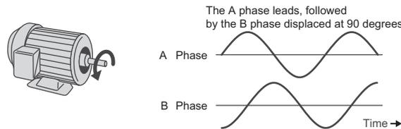
**Figure 59 Displacement of A and B Phases**
