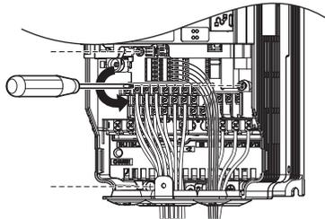
**Figure 88 Drive Replacement: Removing the Control Terminal Board**
