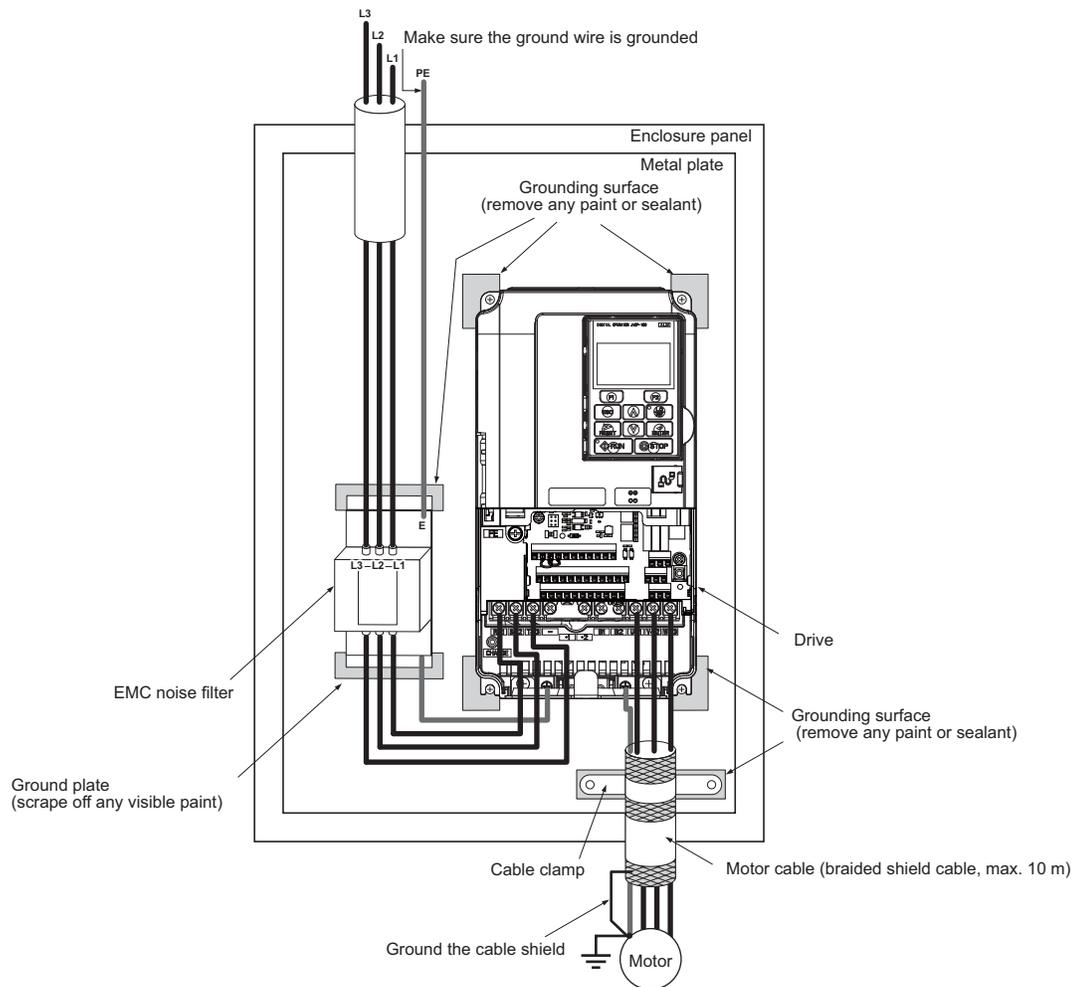
Figure 34 EMC Filter and Drive Installation for CE Compliance (Three-Phase 200 V / 400 V Class)
