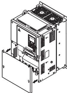
Figure 77 Removing the Terminal Cover
