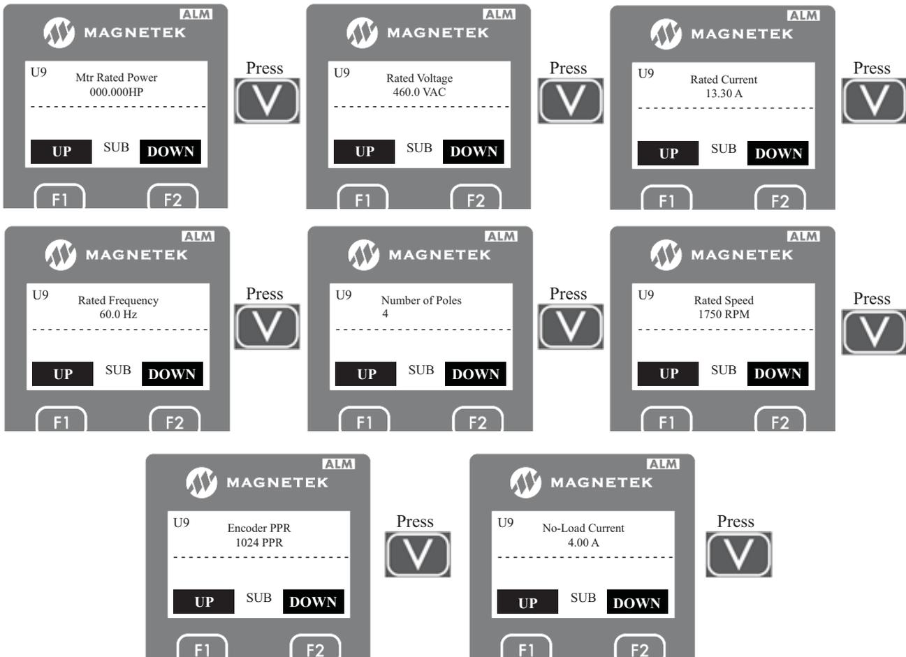
13. After all the data have been entered, the autotune should be initiated by either the “ENTER” key or a RUN signal.
