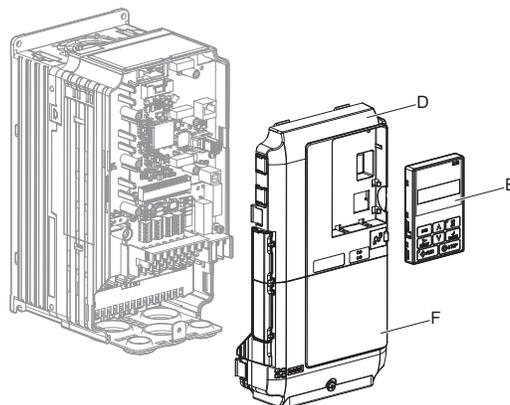
Figure 38 Remove the Front Covers and Digital Operator
