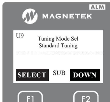
4. On this screen, press the “ENTER” key. Then use the UP or DOWN key to select one of four different types of autotune for induction motors. In this case set it for non-rotational tuning 2 as shown below.
