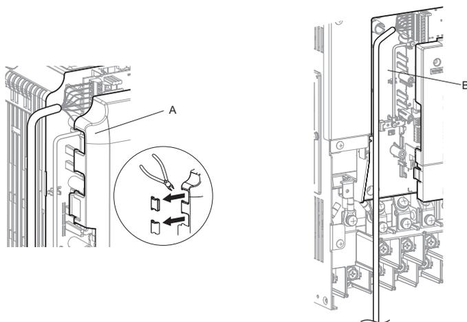
**A – Route wires through the openings provided on the left side of the front cover.**
