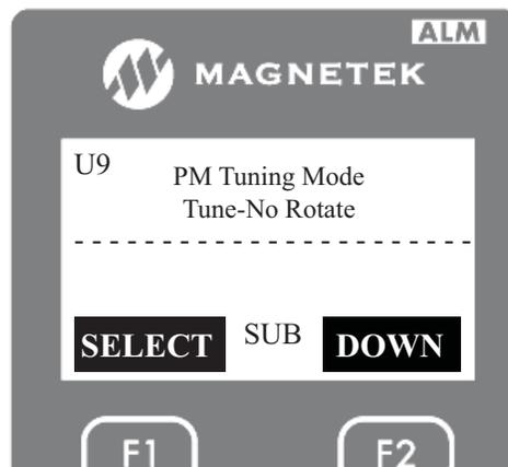
4. On this screen, press the “ENTER” key. Then use the UP or DOWN key to select one of seven different types of autotune for PM motors. In this case set it for terminal resistance as shown below.
