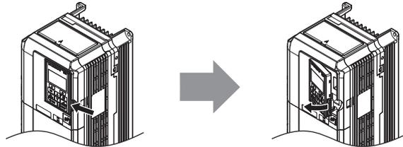
Figure 80 Removing the Digital Operator
