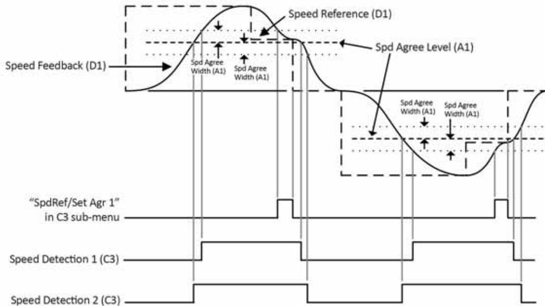
Figure 15 User-set Speed Agree 1, Speed Detection 1, and Speed Detection 2 Timing Diagram
