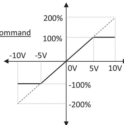
Figure 27 Gain Setting Example
