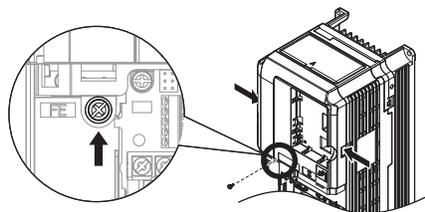
Figure 82 Remove the Front Cover (Models LU2M0018 to 2M0075, 4M0009 to 4M0039, and 5M0003 to 5M0027)
