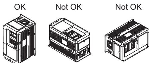
**Figure 71 Correct Installation Orientation**
