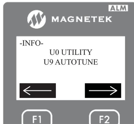
3. Then press the “ENTER” key to access the AUTOTUNE sub-menu screen. The first thing the drive will ask the user is to select a type of autotune as shown below.
