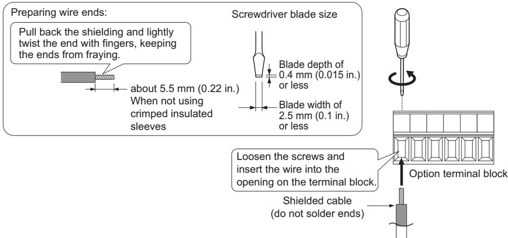
Figure 53 Preparing and Connecting Cable Wiring
