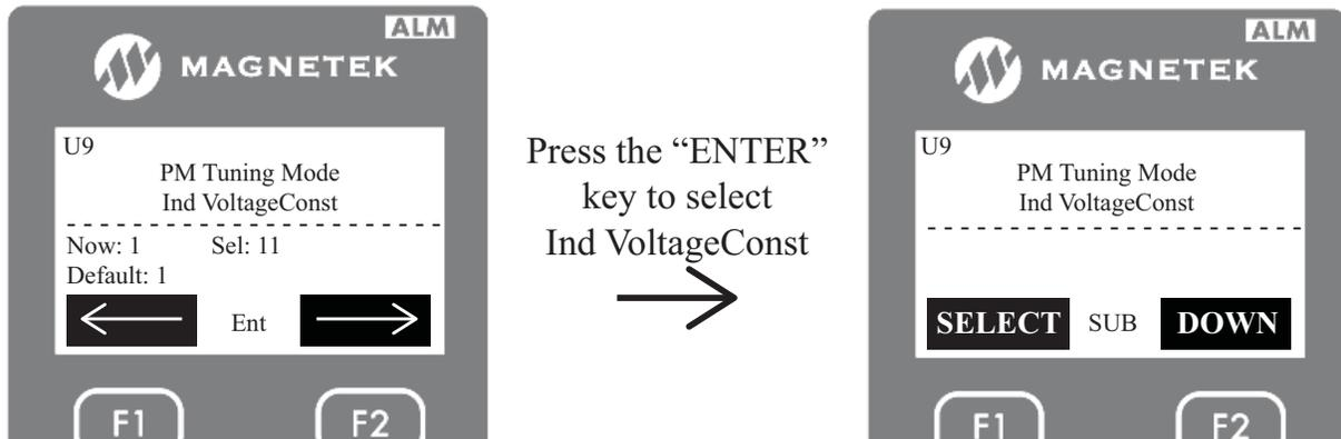
5. After selecting “Ind VoltageConst”, press the DOWN key to begin the autotune.
