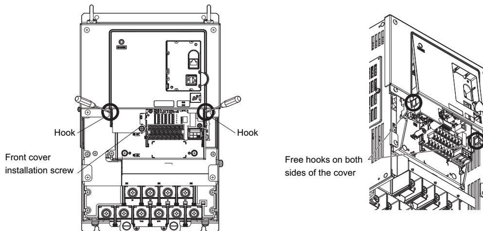
**Figure 83 Remove the Front Cover (Models LU2M0085 to 2M0415, 4M0045 to 4M0216, and 5M0032 to 5M0062)**
