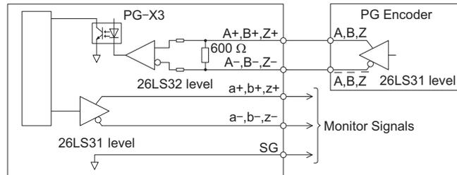
Figure 46 Interface Circuit
