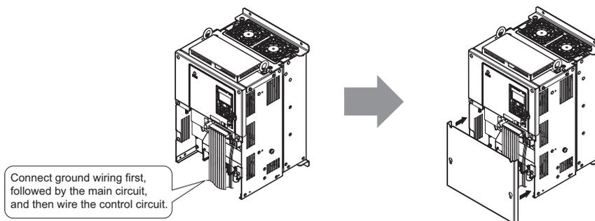
Figure 79 Reattaching the Terminal Cover
