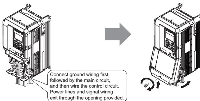
Figure 78 Reattaching the Terminal Cover
