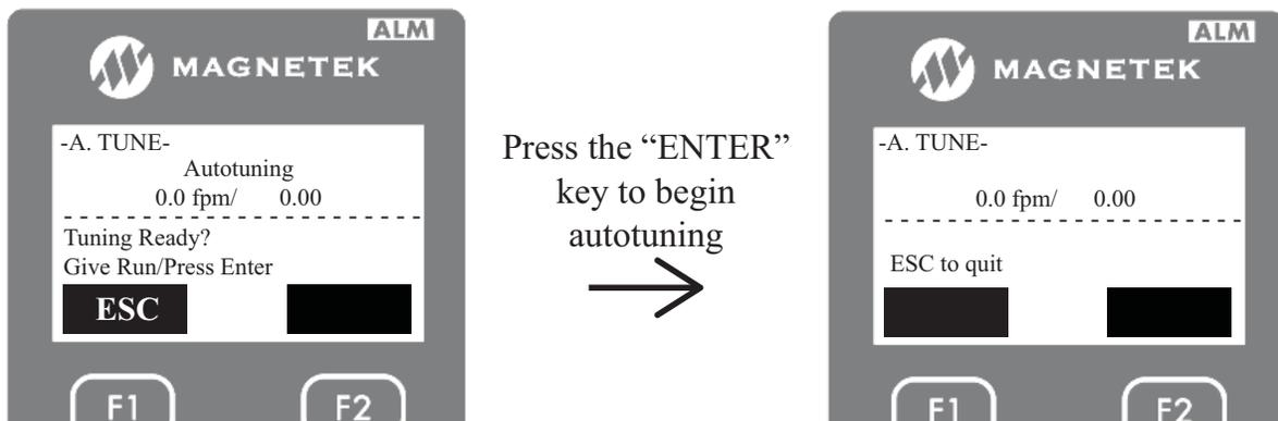
7. During the autotune, the motor will make a noise and start making several turns. After the tuning is done, the drive will announce the following.
