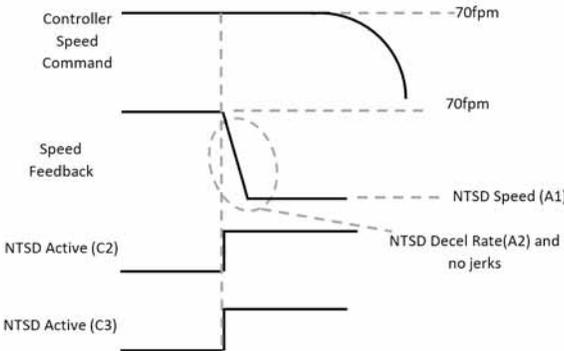
Figure 23 Jerk Disabled NTSD Mode Diagram with NTSD Active Input
