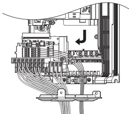
**Figure 89 Drive Replacement: Remove the Control Terminal Board**
