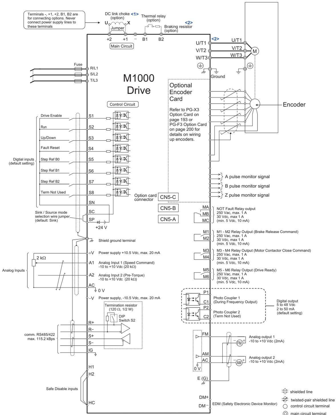
Figure 1 Drive Standard Connection Diagram (example: LU2M0033)
