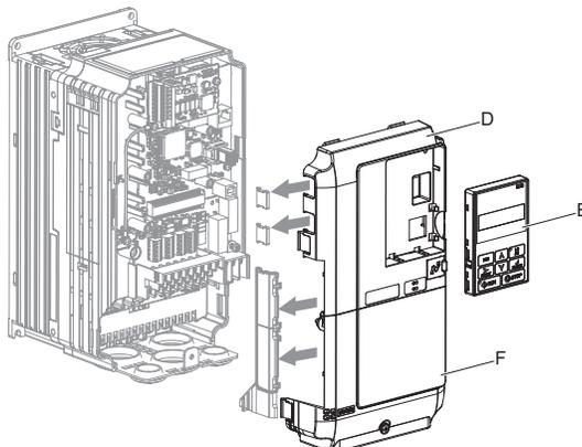
**Figure 43 Replace the Front Covers and Digital Operator**
