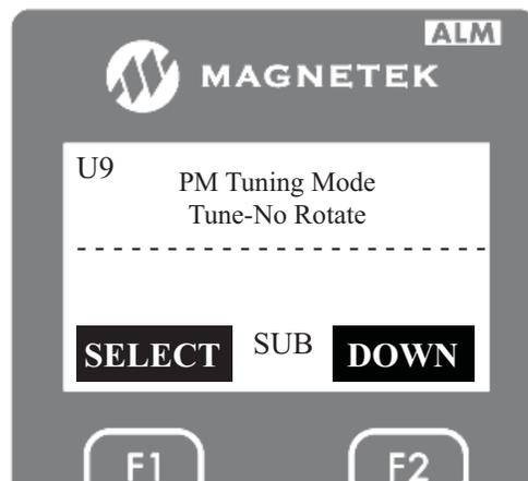
4. On this screen, press the "ENTER" key. Then use the UP or DOWN key to select one of seven different types of autotune for PM motors. In this case set it for the rotor alignment test as shown below.
