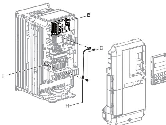
Figure 51 Connect the Ground Wire
