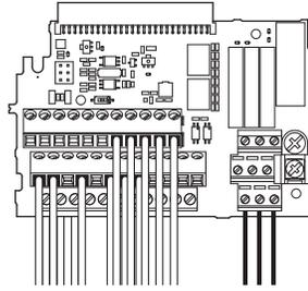
**Figure 90 Drive Replacement: Removable Control Terminal Board Disconnected from the Drive**
