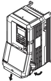
Figure 75 Removing the Terminal Cover
