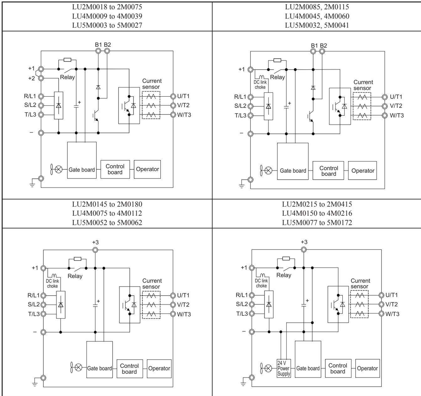
Figure 2 Drive main circuit configurations
