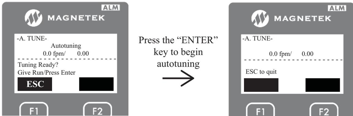
12. During the autotune, the motor will make audible noise and the display will show speed and motor amps as shown above. After the tuning is done, the drive will announce the following.
