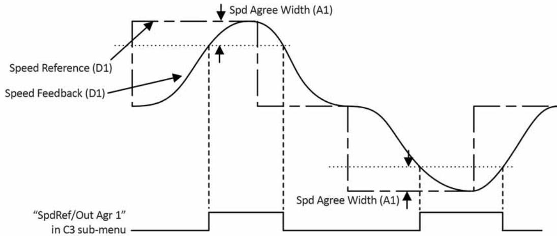
Figure 14 Speed Agree 1 Timing Diagram
