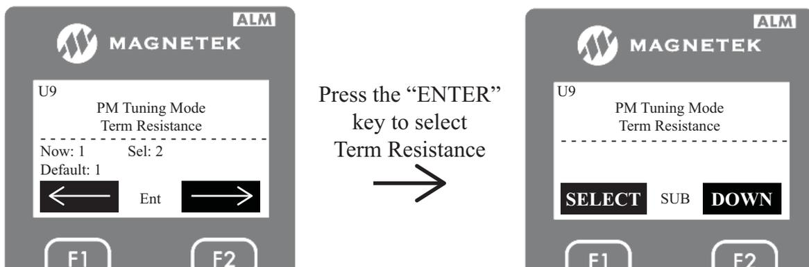
5. After selecting “Term Resistance”, press the DOWN key to enter the next data. The next data the drive will ask the user to enter is the motor nameplate current. The UP key can be pressed to go back to the previous parameter.
