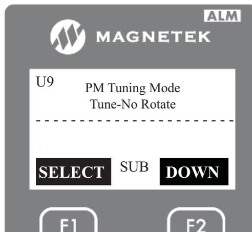
4. On this screen, press the “ENTER” key. Then use the UP or DOWN key to select one of seven different types of autotune for PM motors. In this case set it for non-rotational rotor alignment as show below.
