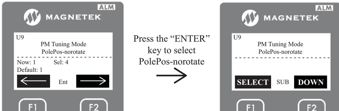
5. After selecting “PolePos-norotate”, press the DOWN key to begin the non-rotational rotor alignment.
