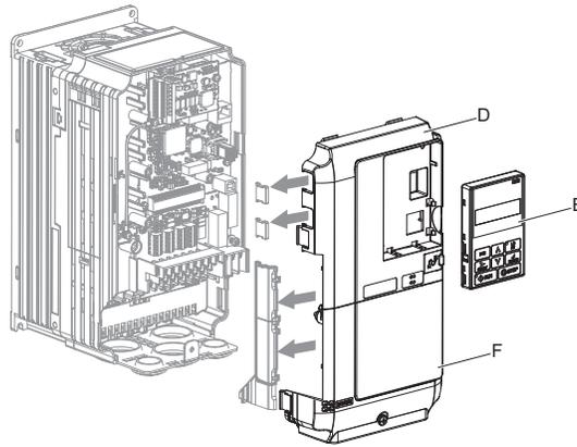
**Figure 58 Replace the Front Covers and Digital Operator**
