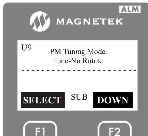
4. On this screen, press the “ENTER” key. Then use the UP or DOWN key to select one of seven different types of autotune for PM motors. In this case set it for rotational rotor alignment as show below.
