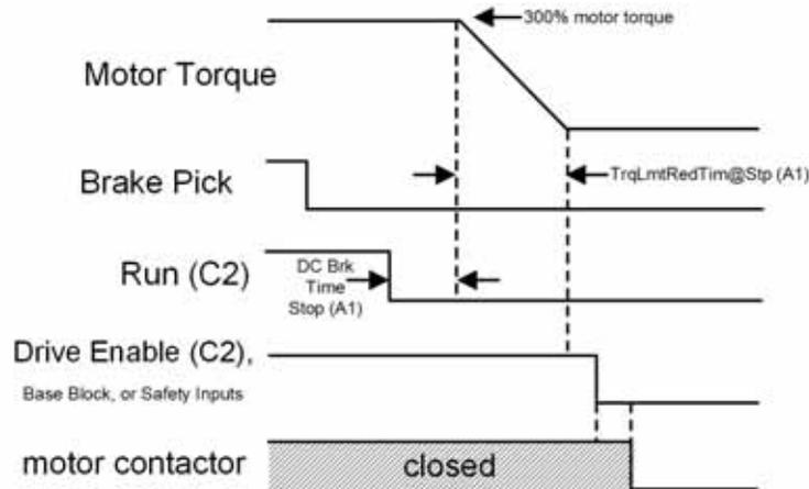
Figure 11 Torque Ramp Down Timing Diagram
