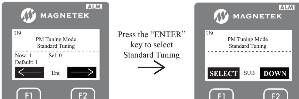
5. After selecting “Standard Tuning”, press the DOWN key to enter the next data. The next data the drive will ask the user to enter is the motor nameplate power in horsepower.
