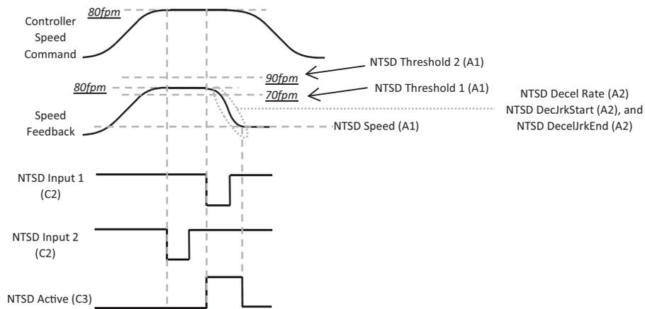
Figure 20 Two Thresholds NTSD Mode Diagram
