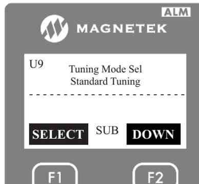
4. On this screen, press the “ENTER” key. Then use the UP or DOWN key to select one of four different types of autotune for induction motors. In this case set it for terminal resistance as shown below.
