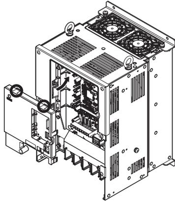
Figure 85 Reattach the Front Cover (Models LU2M0085 to 2M0415, 4M0045 to 4M0216, and 5M0032 to 5M0062)
