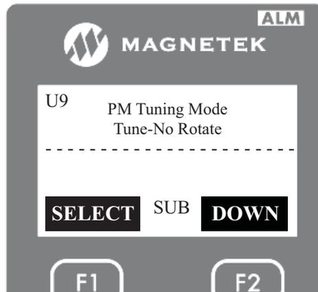
4. On this screen, press the “ENTER” key. Then use the UP or DOWN key to select one of seven different types of autotune for PM motors. In this case set it for standard tuning, as shown below.
