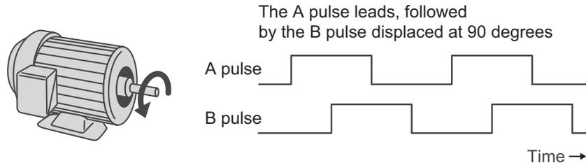
**Figure 44 Displacement of A and B Pulses**
