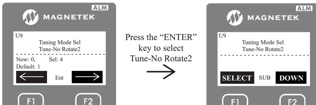
5. After selecting “Tune-No Rotate2”, press the DOWN key to enter the next data. The next data the drive will ask the user to enter is the motor nameplate power in horsepower.
