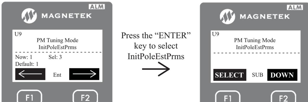
5. After selecting "InitPoleEstPrms", press the DOWN key to begin the rotor alignment test.
