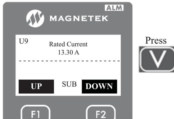
6. After all the data have been entered, the autotune should be initiated by either the “ENTER” key or a RUN signal.
