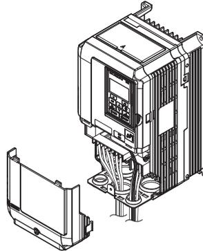
**Figure 87 Drive Replacement: Removing the Terminal Cover**
