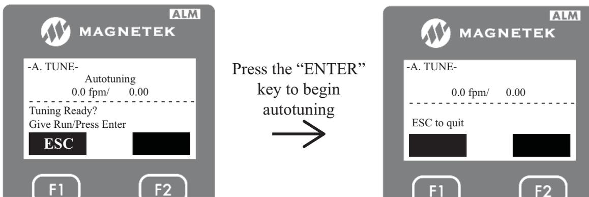
7. During the alignment test, the motor will make audible noise and the display will show speed and motor amps as shown above. After the test is done, the drive will announce the following.
