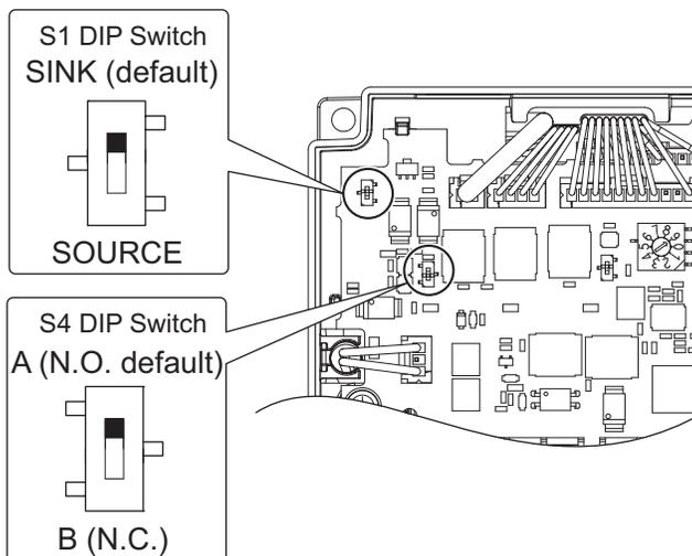
Figure 65 Setting CDBR Onboard DIP Switches
