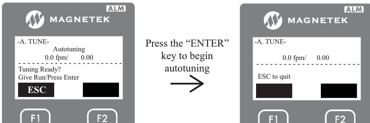
7. During the autotune, the motor will make audible noise and the display will show speed and motor amps as shown above. After the tuning is done, the drive will announce the following:
