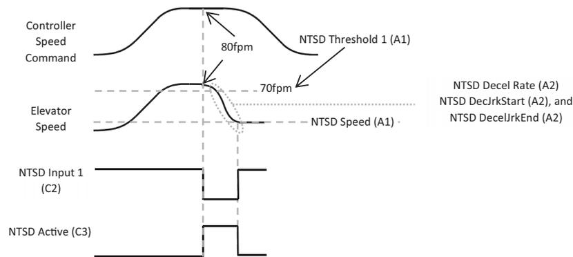
Figure 19 One Threshold NTSD Mode Diagram
