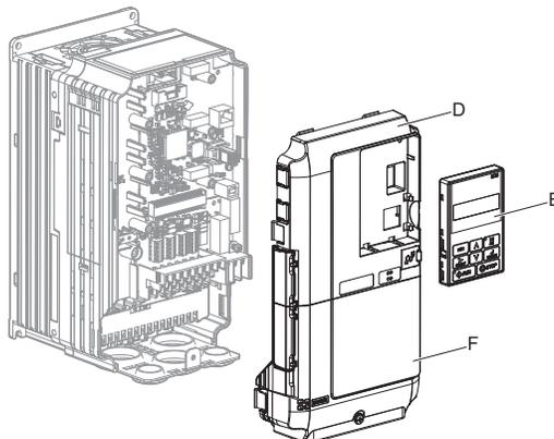
Figure 49 Remove the Front Cover, Terminal Cover, and Digital Operator
