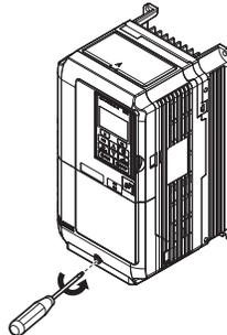
Figure 74 Removing the Terminal Cover
