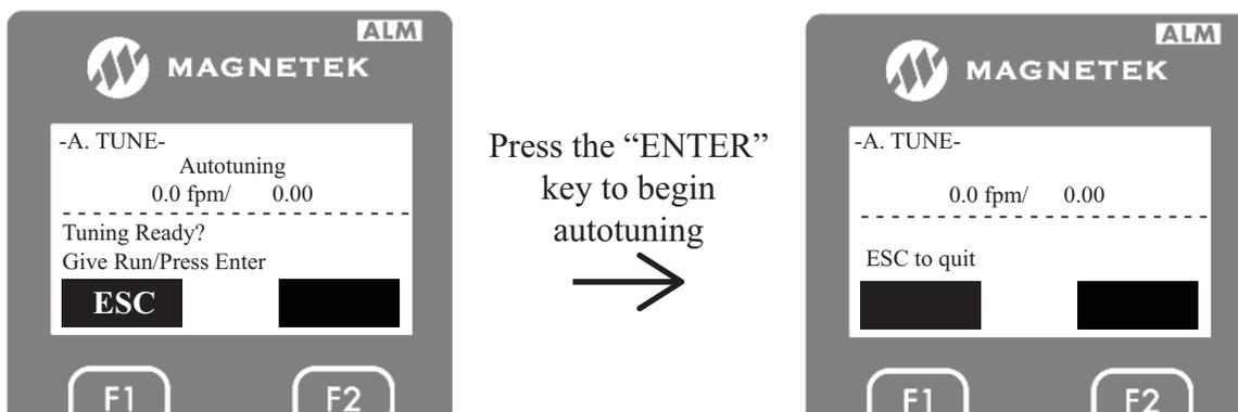
15. During the autotune, the motor will make audible noise and the display will show speed and motor amps as shown above. After the tuning is done, the drive will announce the following:
