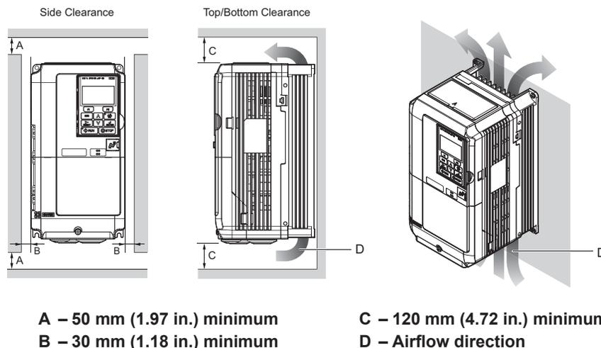
Figure 72 Correct Installation Spacing
