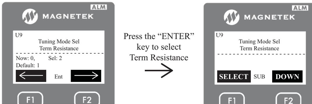
5. After selecting “Term Resistance”, press the down key to enter the next data. The next data the drive will ask the user to enter is the motor nameplate power in horsepower.
