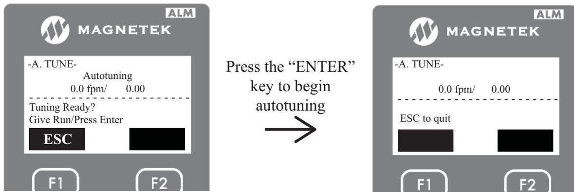
8. During the autotune, the motor will make audible noise and the display will show speed and motor amps as shown above. After the tuning is done, the drive will announce the following:
