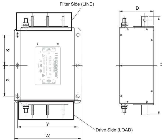
Figure 35 EMC Filter Dimensions
