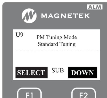
4. On this screen, press the "ENTER" key. Then use the UP or DOWN key to select one of seven different types of autotune for PM motors. In this case set it for tuning no rotation as shown below.
