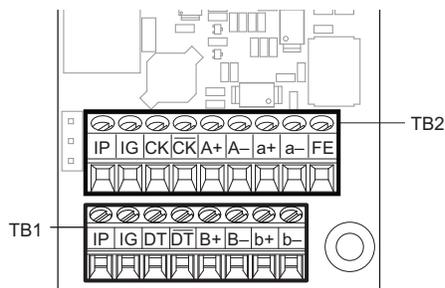
Refer to [Table 92 on page 210](#) and [Table 93 on page 211](#) for details on TB1 and TB2 terminal functions and signal levels.
