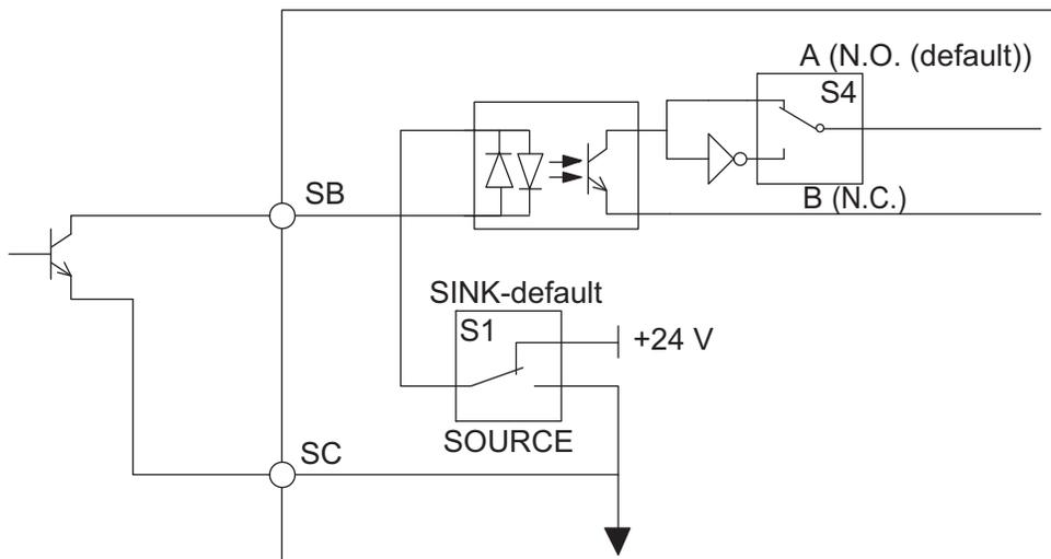
Figure 66 CDBR Braking Unit Sinking Mode using Internal Power Supply
