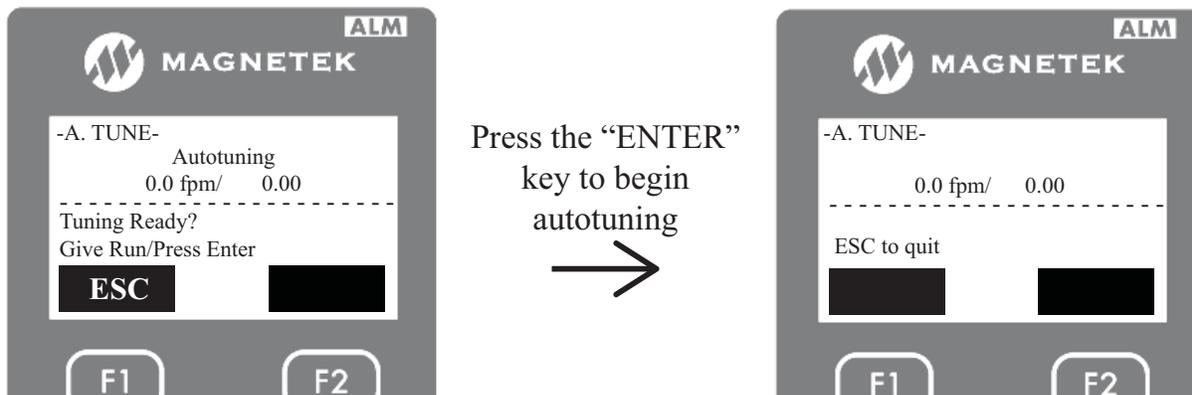
7. During the alignment, the motor will make a noise and jerk. Then it will stop and jerk again in the opposite direction. After the alignment is done, the drive will announce the following.
