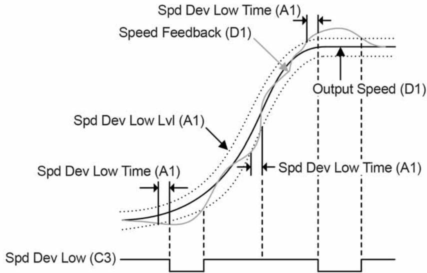
Figure 13 Speed Deviation Low Timing Diagram
