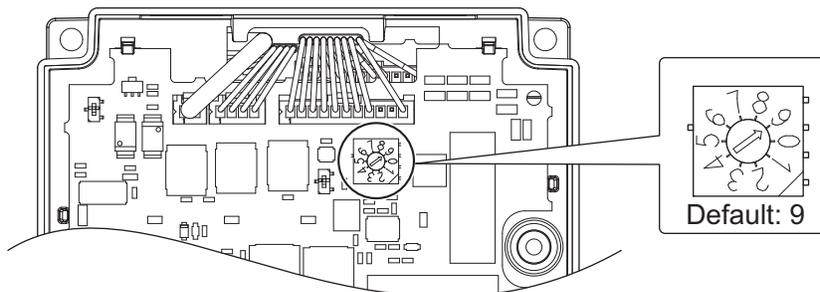
Figure 69 CDBR Voltage Activation Level, Rotary Switch (S3)
