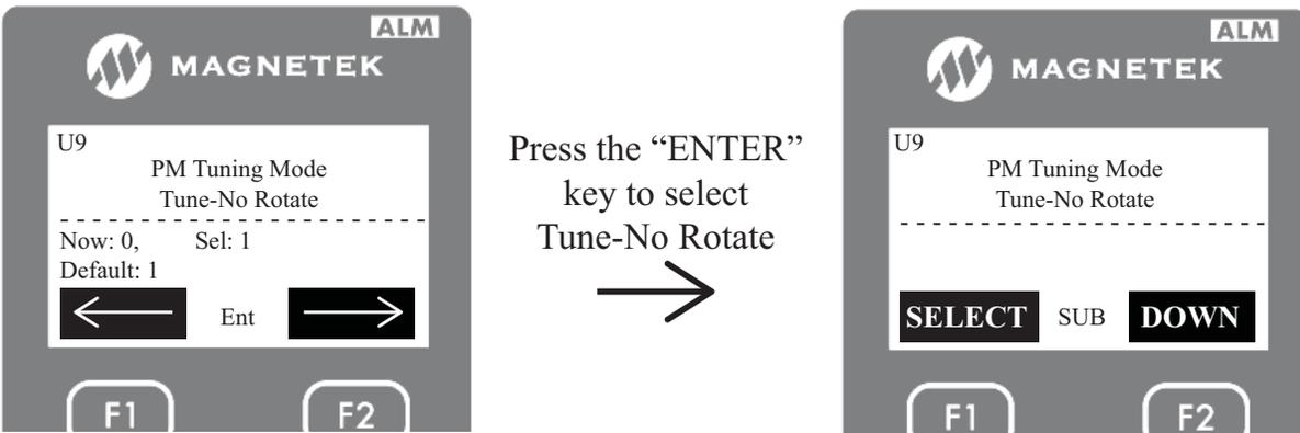
5. After selecting “Tune-No Rotate”, press the DOWN key to enter the next data. The next data the drive will ask the user to enter is the motor nameplate power in horsepower.
