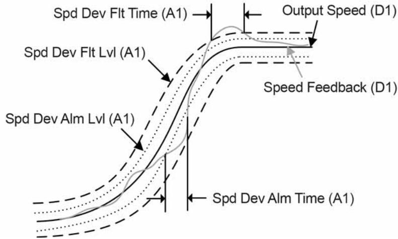
Figure 12 Speed Deviation Alarm and Fault
