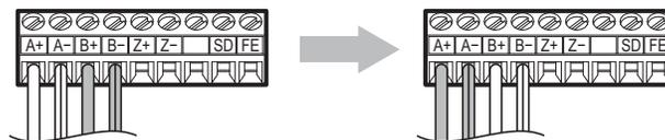
**Figure 45 A Channel and B Channel Wire Switching**
