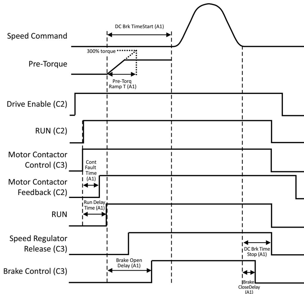
**Figure 29 Timing Diagram for Drive Ramp to Stop**
