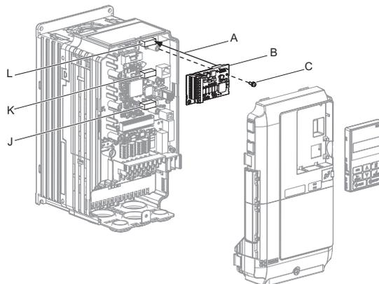
**Figure 39 Insert the Option and Connect the Ground Wire**
