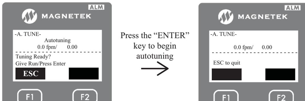
14. During the autotune, the motor will make audible noise and the display will show speed and motor amps as shown above. After the tuning is done, the drive will announce the following.
