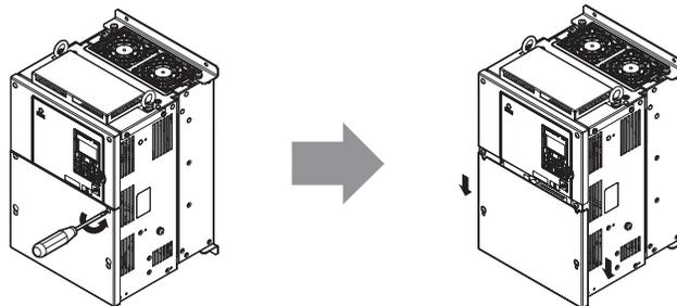
Figure 76 Removing the Terminal Cover
