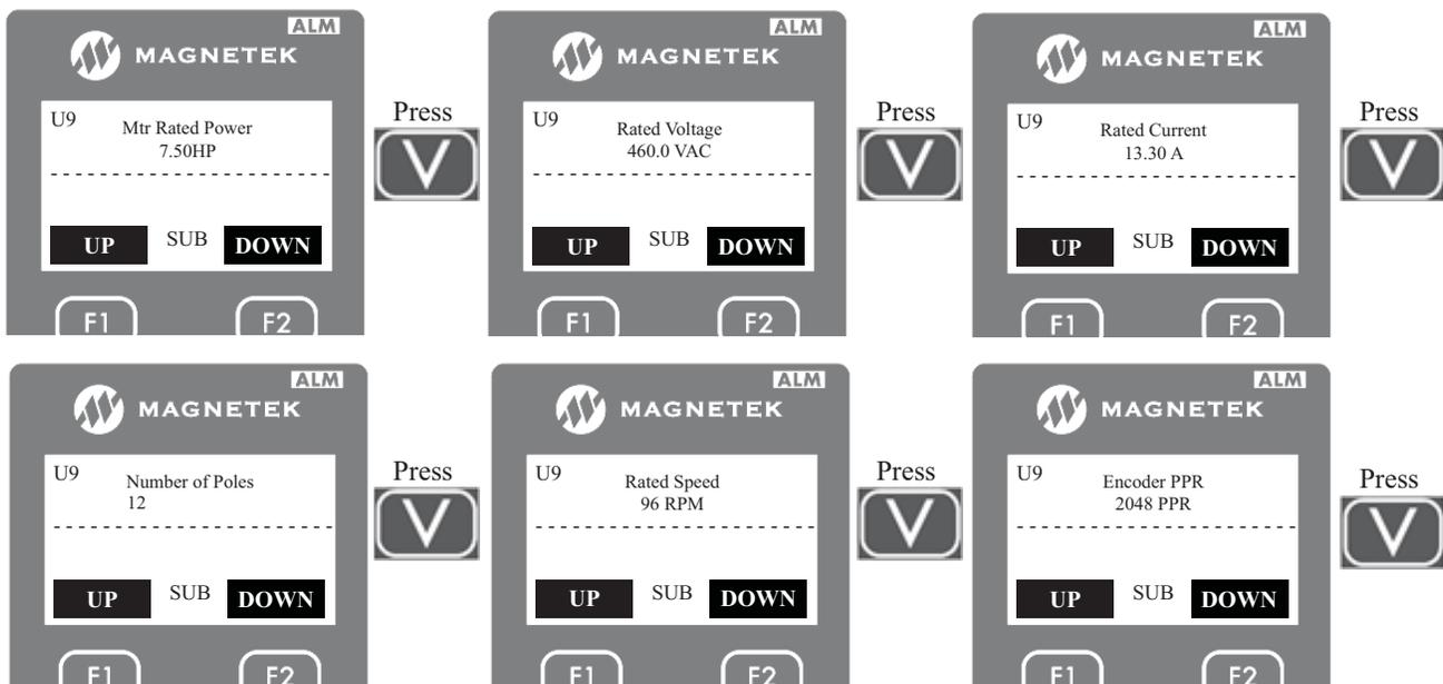
11. After all the data have been entered, the autotune should be initiated by either the “ENTER” key or a RUN signal.
