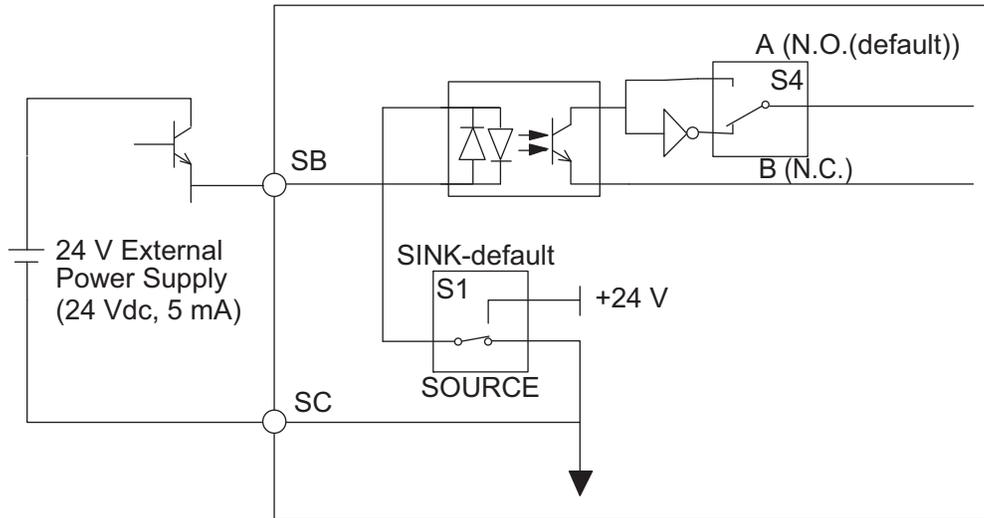
**Figure 67 CDBR Braking Unit Sourcing Mode**
