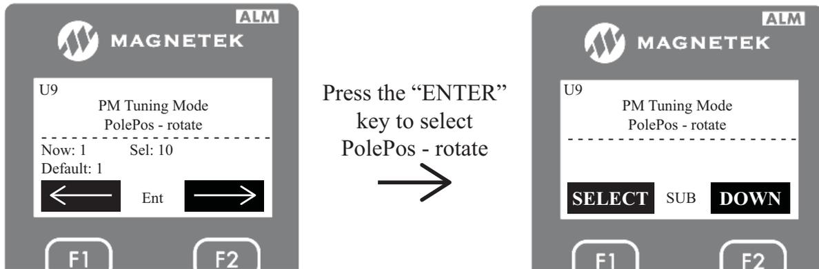
5. After selecting “PolePos - rotate”, press the DOWN key to begin the rotational rotor alignment.
