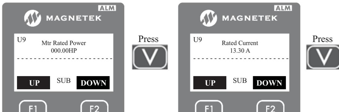
7. After all the data have been entered, the autotune should be initiated by either the “ENTER” key or a RUN signal.
