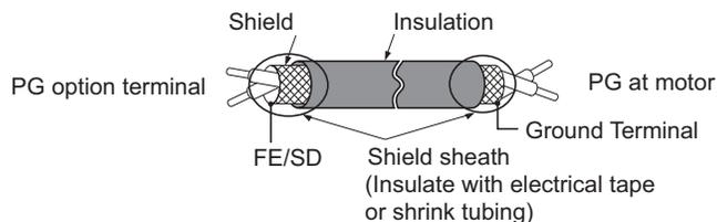
Figure 52 Preparing Ends of Shielded Cable
