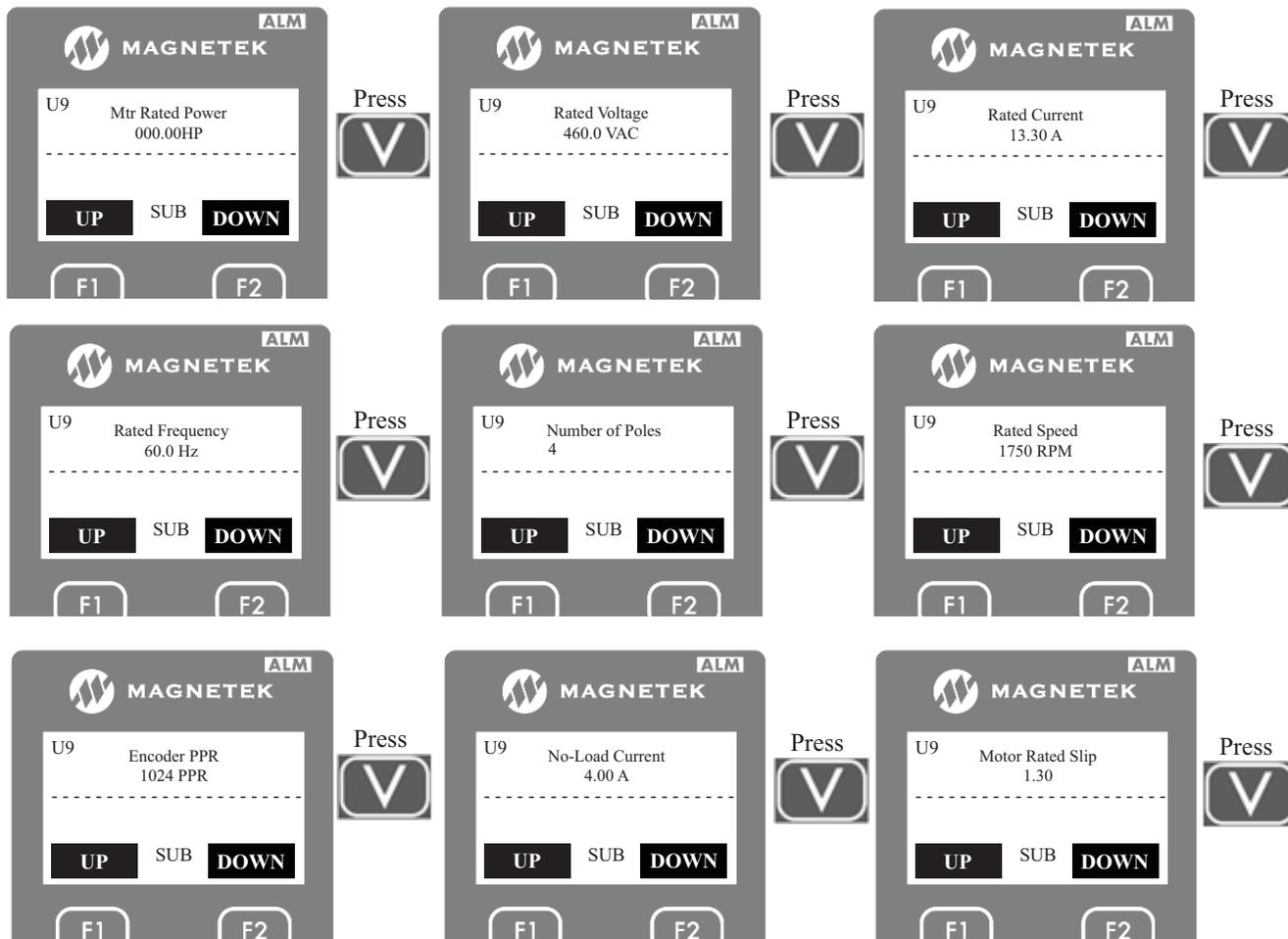
14. After all the data have been entered, the autotune should be initiated by either the “ENTER” key or a RUN signal.
