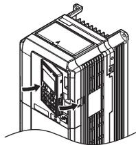
Figure 81 Reattaching the Digital Operator
