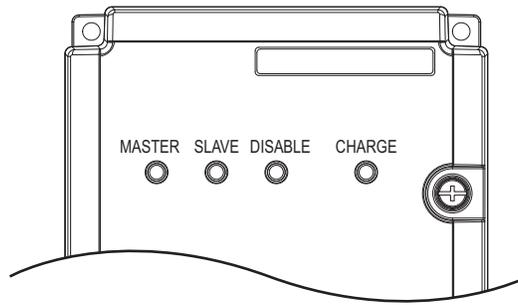
Figure 64 CDBR Braking Unit LED Display
