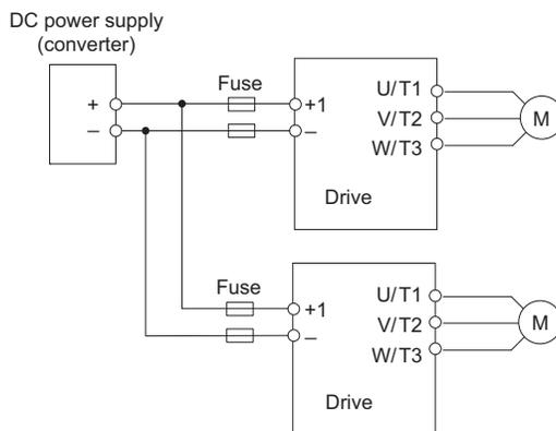
**Figure 31 Example of DC Power Supply Input (two M1000 drives connected in series)**
