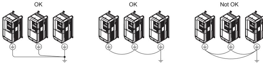
Figure 73 Multiple Drive Wiring
