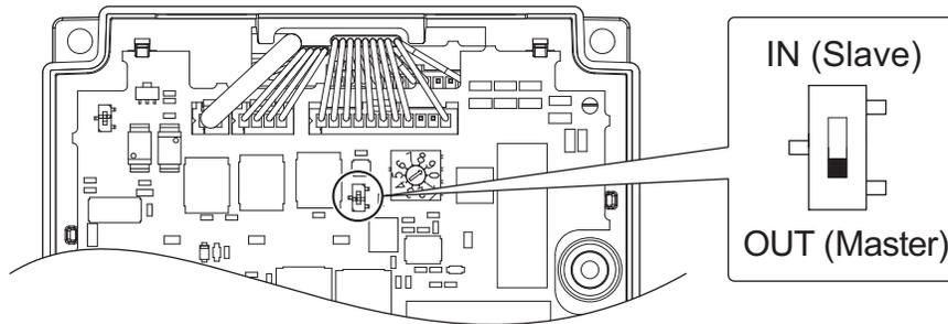
**Figure 68 Master/Slave Selection Switch (S2)**
