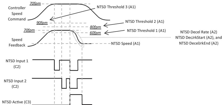
Figure 21 Three Thresholds NTSD Mode Diagram
