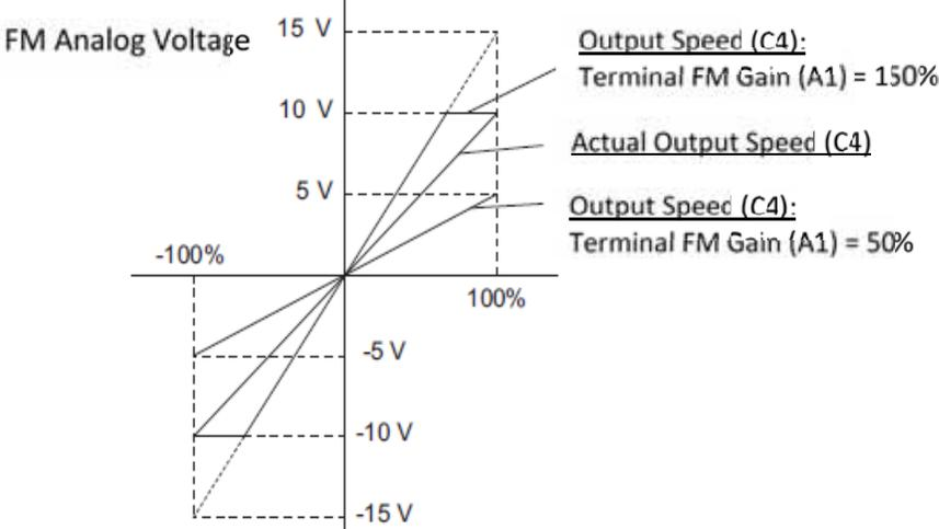
Figure 26 Gain Setting Example
