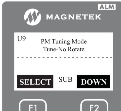
4. On this screen, press the “ENTER” key. Then use the UP or DOWN key to select one of seven different types of autotune for PM motors. In this case set it for inductance voltage constant as show below.
