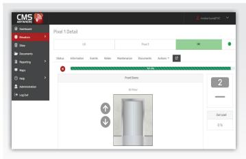
With EMU Gateway on Pixel and GALaxy controls, calls can be placed onto elevators from anywhere in the world. The service provider can interrogate the elevator status, verify faults and reduce costly site visits by remote fault verification.
