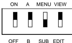
3. Move the VIEW/EDIT DIP switch back to the position shown. To select another Parameter in the selected sub-menu, use the UP and DN push buttons. To select another User Display sub-menu, start over again as on the previous page.
