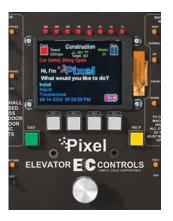
Save time with the intuitive Touch & Go™ on-board user interface, available at three points of access (machine room, inside cab, cab top)
