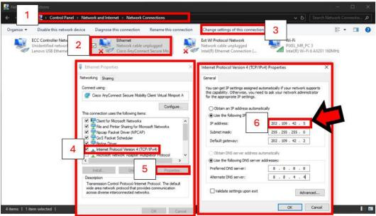
2. Configure the testing PC network adapter by opening the same Network Connections window shown in the last step to set the IP address the same as the machine room PC with the last number in the IP address increased by one. The subnet will be the same and other settings are left blank.
