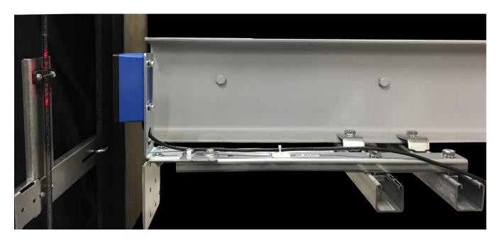
Figure E1.7: CEDES APS Camera Mounting Bracket
