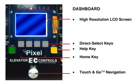
Figure i1 - System Access Point
