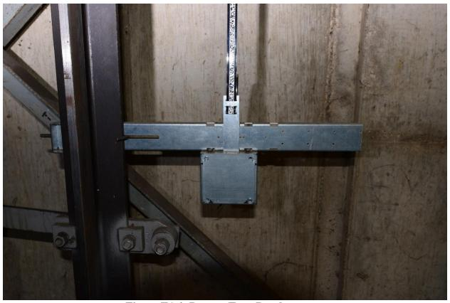
Figure E1.4: Bottom Tape Bracket
