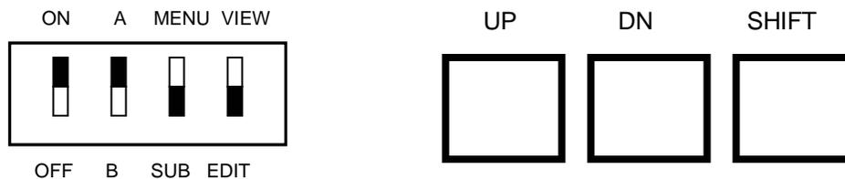
1. Set the DIP switches as shown to change a User Display parameter. Use the UP, DN and SHIFT push buttons to change the value of the parameter.
