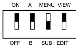
3. Move the **VIEW/EDIT** DIP switch back to the position shown. To select another Parameter in the selected sub-menu, use the **UP** and **DN** push buttons. To select another User Display submenu, start over again as on the previous page.
