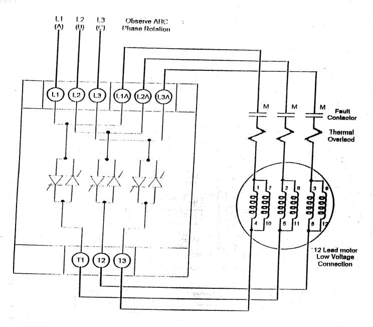
Size wire, contactor and thermal overload for motor leg current, not total phase current. Leg current = phase current x 0.58.
