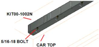
Mount the top angle to the bottom angle using (4) 5/16-18 bolts.
