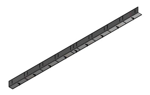
KIT00-1001N is designed to be able to mount GAL headers of any length. 5/16-18 holes are spaced 10" apart for the GAL haeder to be attached. Slots are cut periodicly down the length of the bracket to allow for it to be cut down in the field easily if needed.
