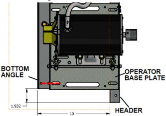
Drill and tap (4) 5/16-18 holes to mount the bottom angle to the cartop.
