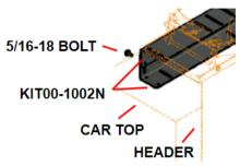
For Config. B, the top angle will have the flange with tapped holes facing downward and flush with the upright bottom flange.
