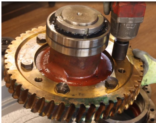
Figure 4-43: Remove Bolts and Nuts From Gear
