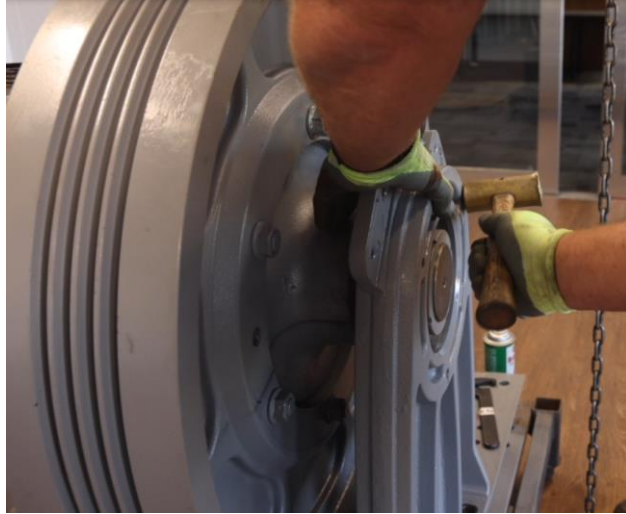
Figure 4-98: Tap the Outboard Stand Into Location Using Brass Hammer
