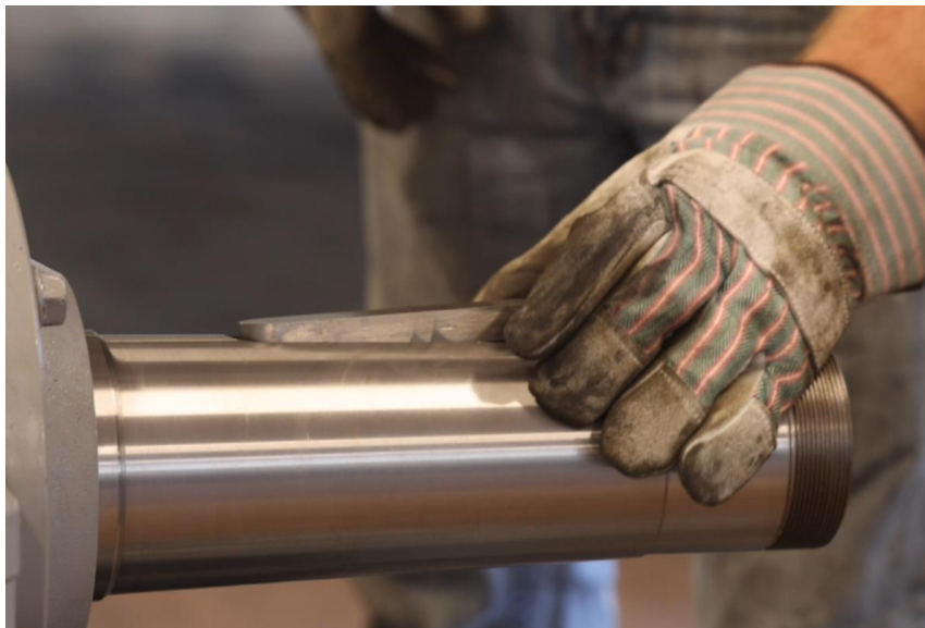
Figure 4-89: Reinstall Original Shaft Key
