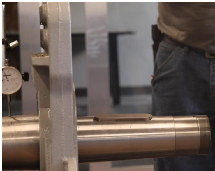
Figure 4-136: Thoroughly Clean Exposed End of Shaft
