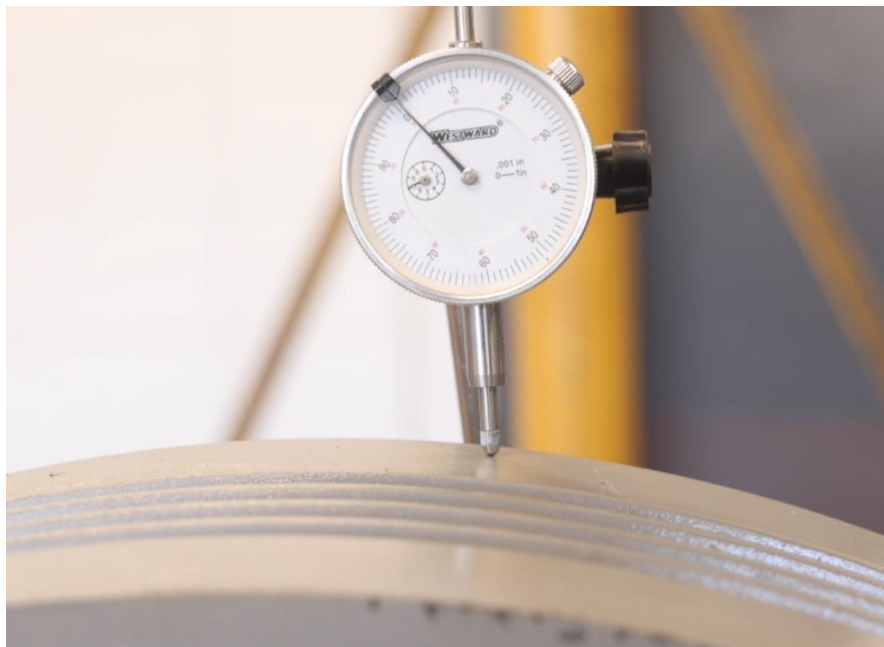
Figure 4-102: Set Indicator to Zero
