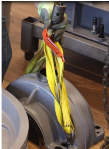
Figure 4-75: Install Eyebolts and Straps to Upper Housing
