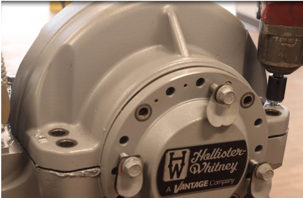
Figure 4-32: Use the Jack Bolts to Separate the Upper and Lower Housing
