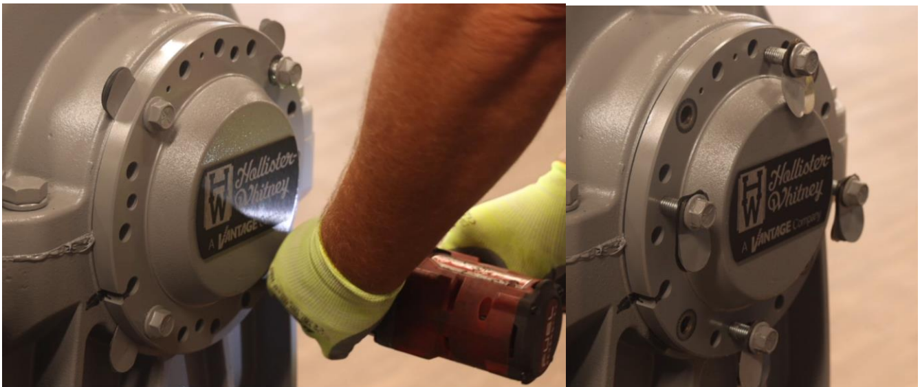
Figure 4-29: Remove Bolts and Shims and Reinstall in Threaded Holes As Shown (with shims)
