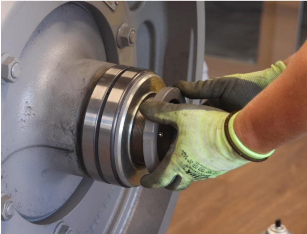
Figure 4-143: Install Shaft Lock Nut Until Snug
