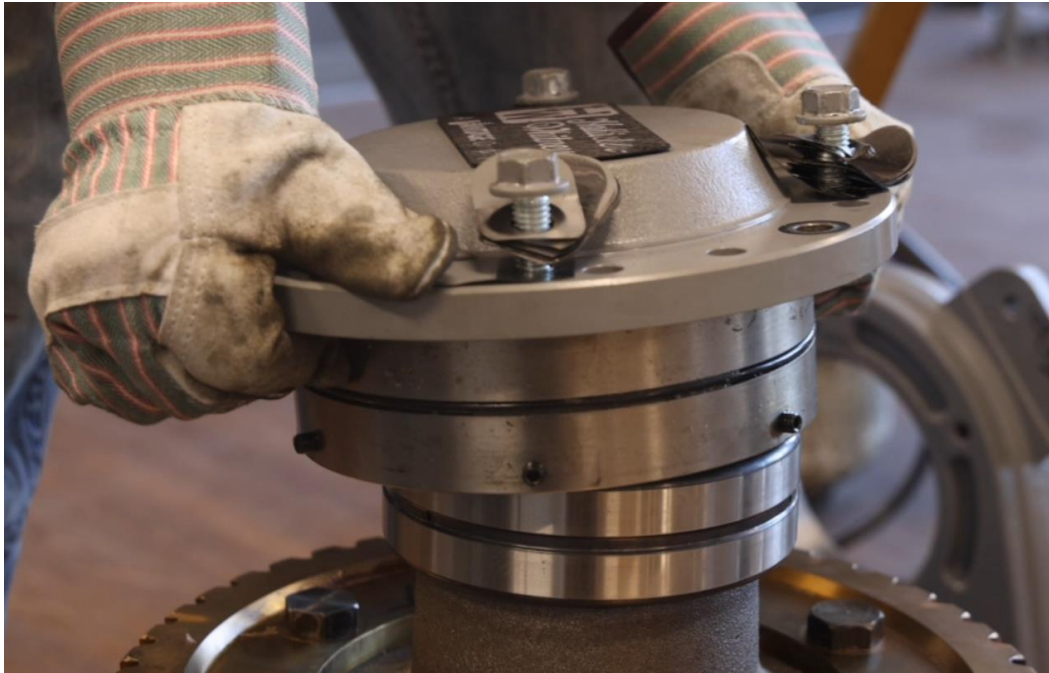
Figure 4-62: Install the Eccentric
