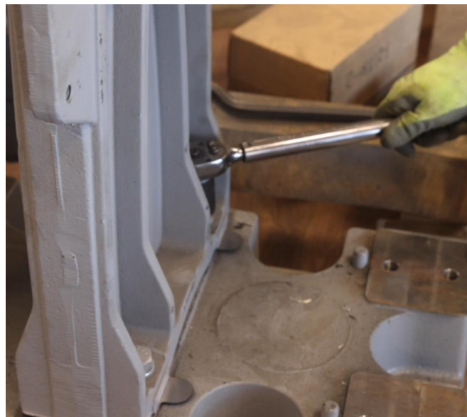
Figure 4-130: Tighten the Four Inner Outboard Stand Bolts
