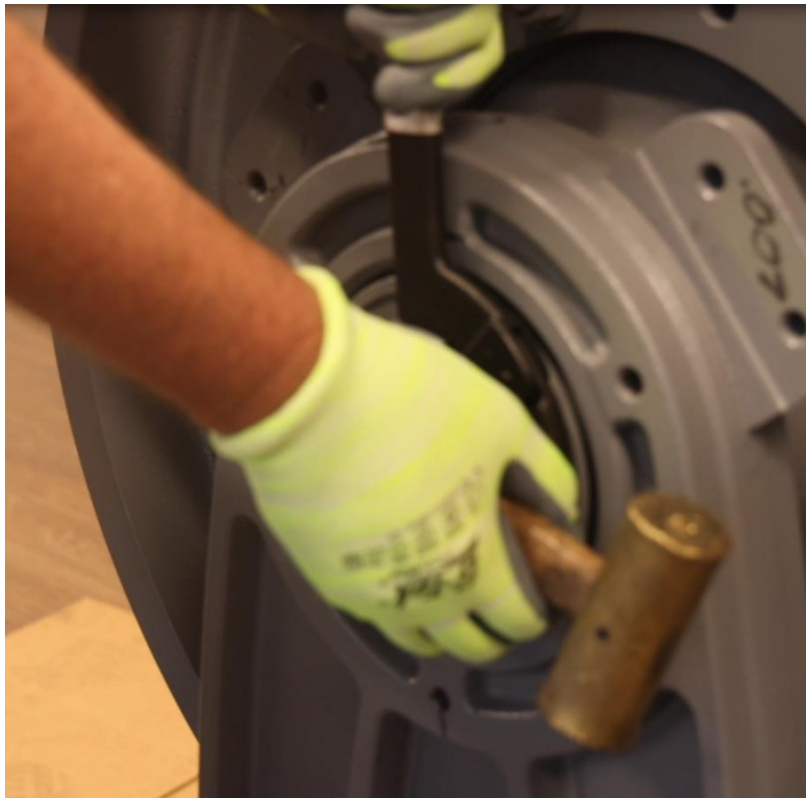
Figure 4-11: Remove Shaft Lock Nut
