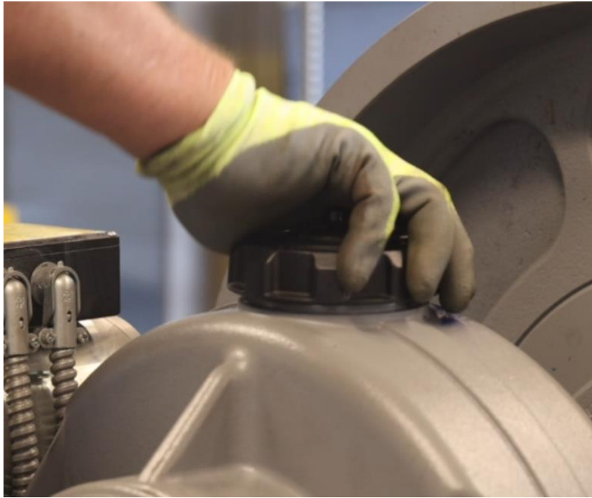
Figure 4-167: Reinstall Oil Cap
