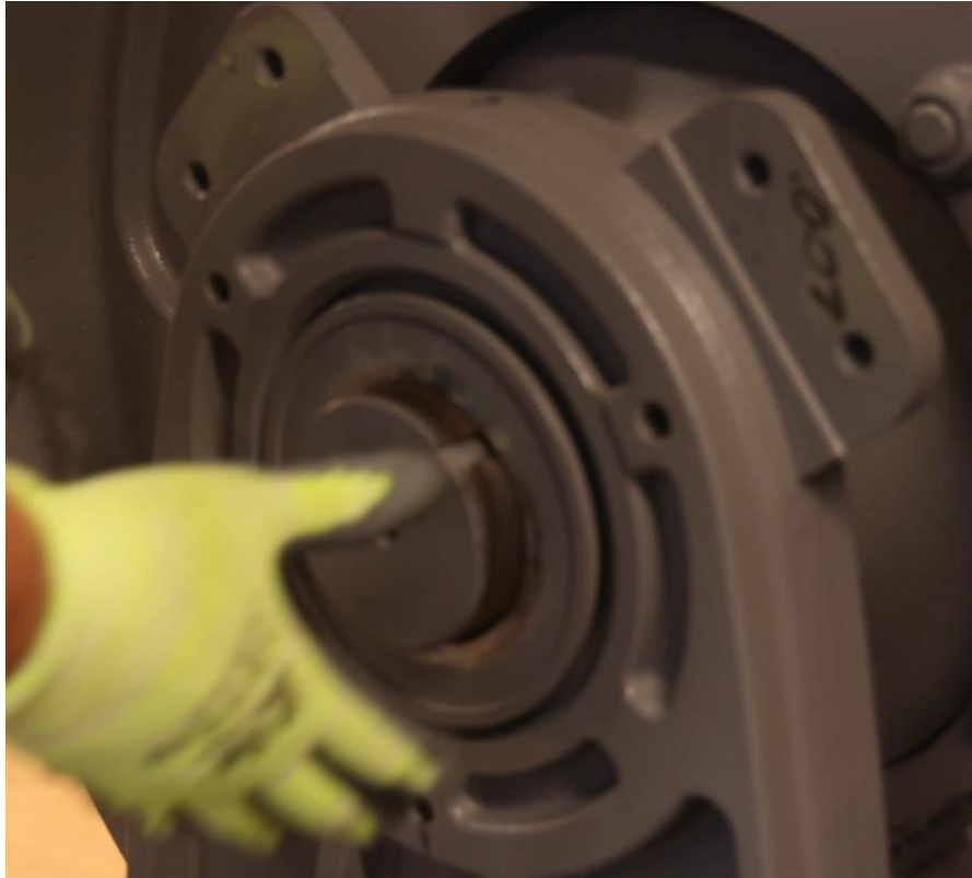
Figure 4-12: Remove Shaft Lock Nut Washer
