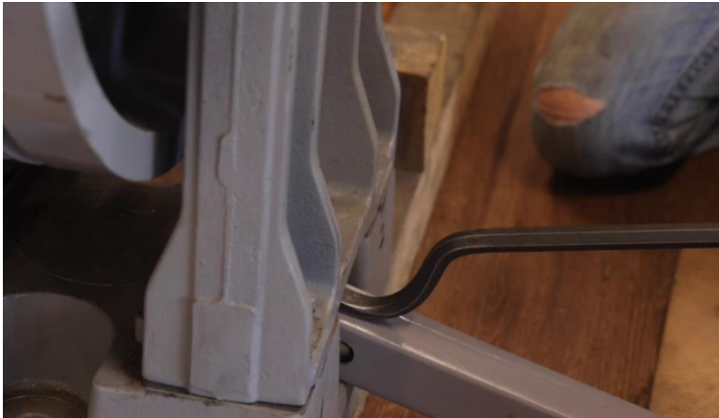
Figure 4-154: Pry Up on Outer Outboard Stand
