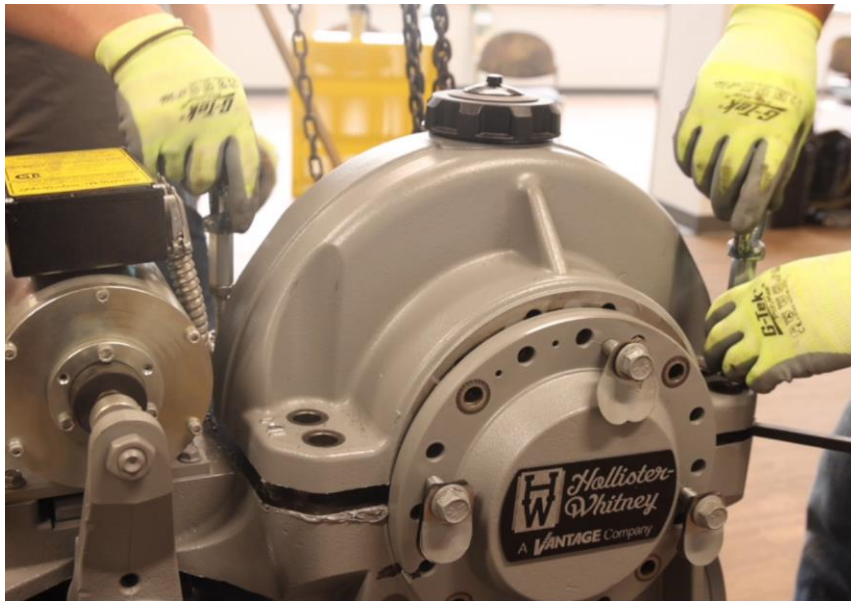
Figure 4-34: Use the Jack Bolts to Separate the Upper and Lower Housing
