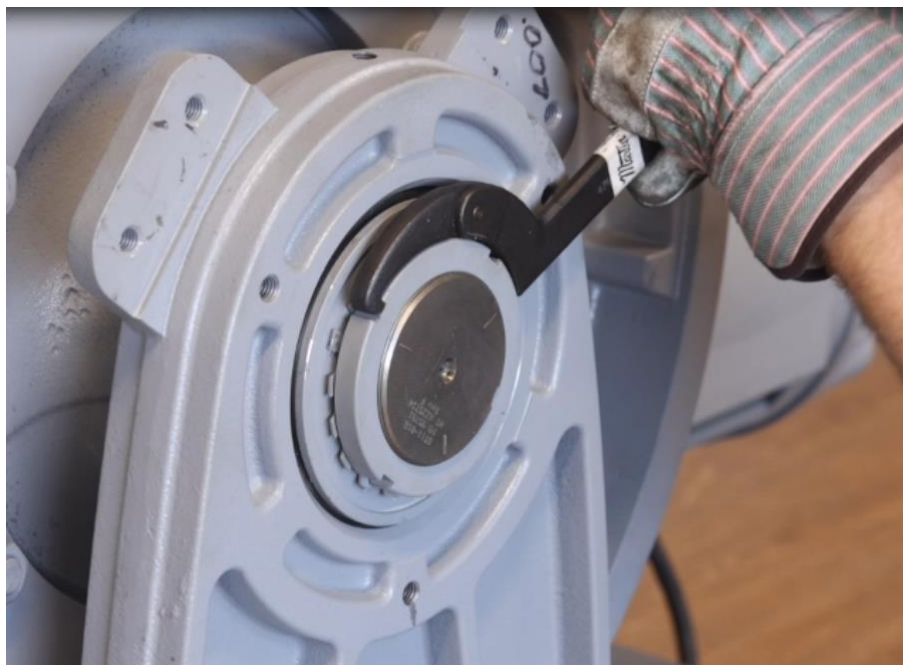
Figure 4-116: Fully Tighten Shaft Lock Nut
