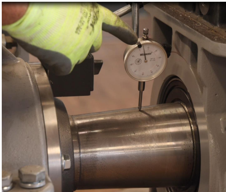
Figure 4-128: Add Enough Shims to Get Appropriate Dial Indicator Reading
