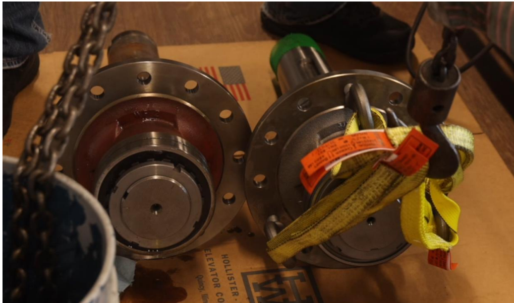
Figure 4-49: Place Hoisting Strap on New Center Assembly
