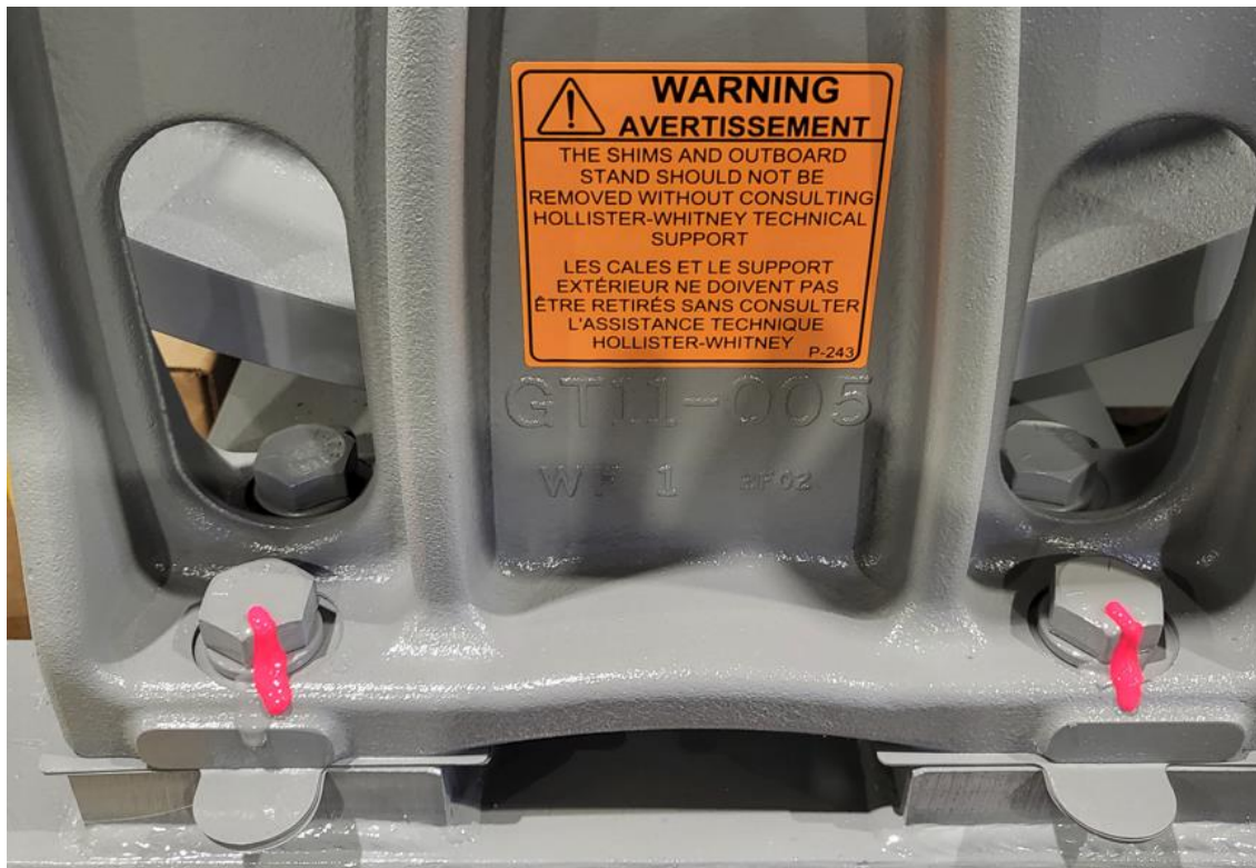
Figure 4-169: Add Orange Warning Label Where Shown
