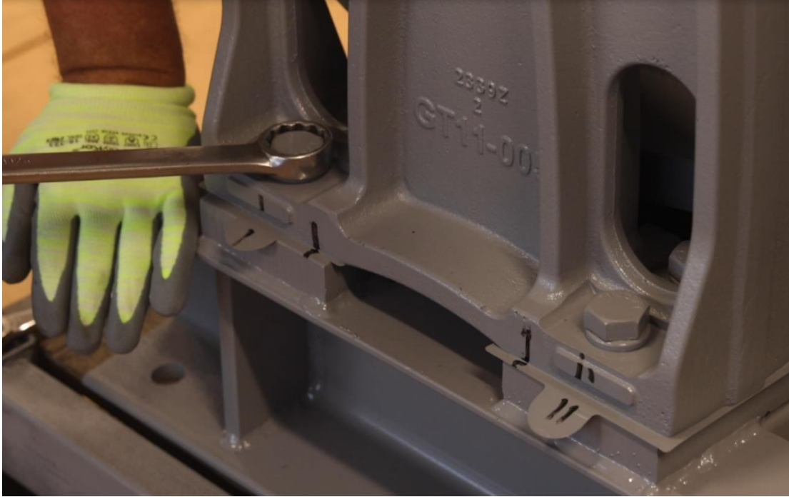
Figure 4-17: Remove Four Bearing Stand Bolts
