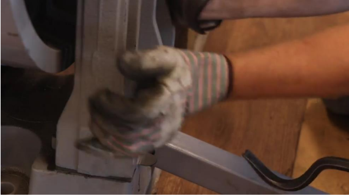
Figure 4-159: Shim Pack Should Be Tight Enough So That There is No Rocking Back and Forth
