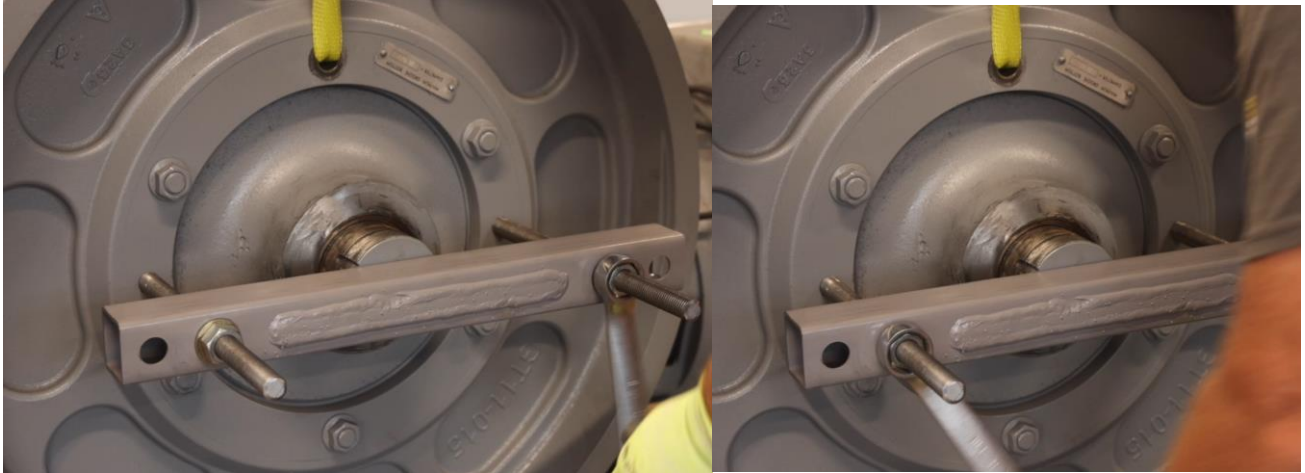
Figure 4-24: Use Puller Assembly To Disengage Traction Wheel Hub from Shaft
