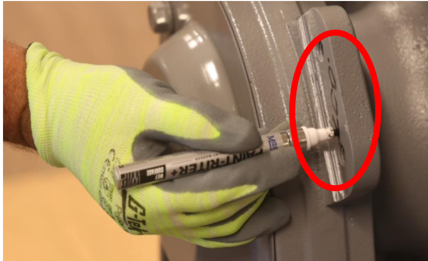
Figure 4-2: Record Backlash on Tab
