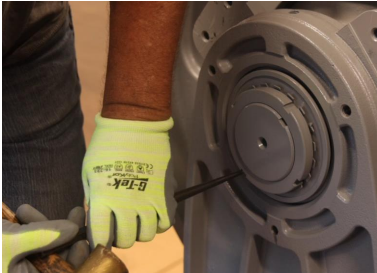
Figure 4-10: Bend Lock Tab Out of Slot in Lock Nut
