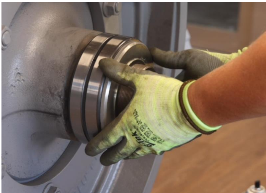
Figure 4-142: Reinstall Original Outboard Stand Bearing
