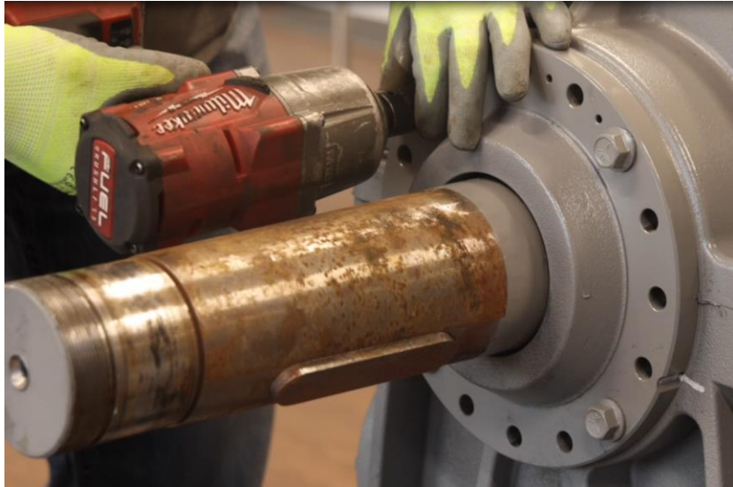
Figure 4-28: Remove All Traction Wheel Side Eccentric Bolts
