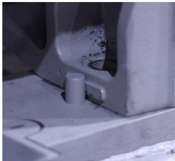
Figure 4-110: Both Dowel Pins In Base Should Be Against Outboard Stand
