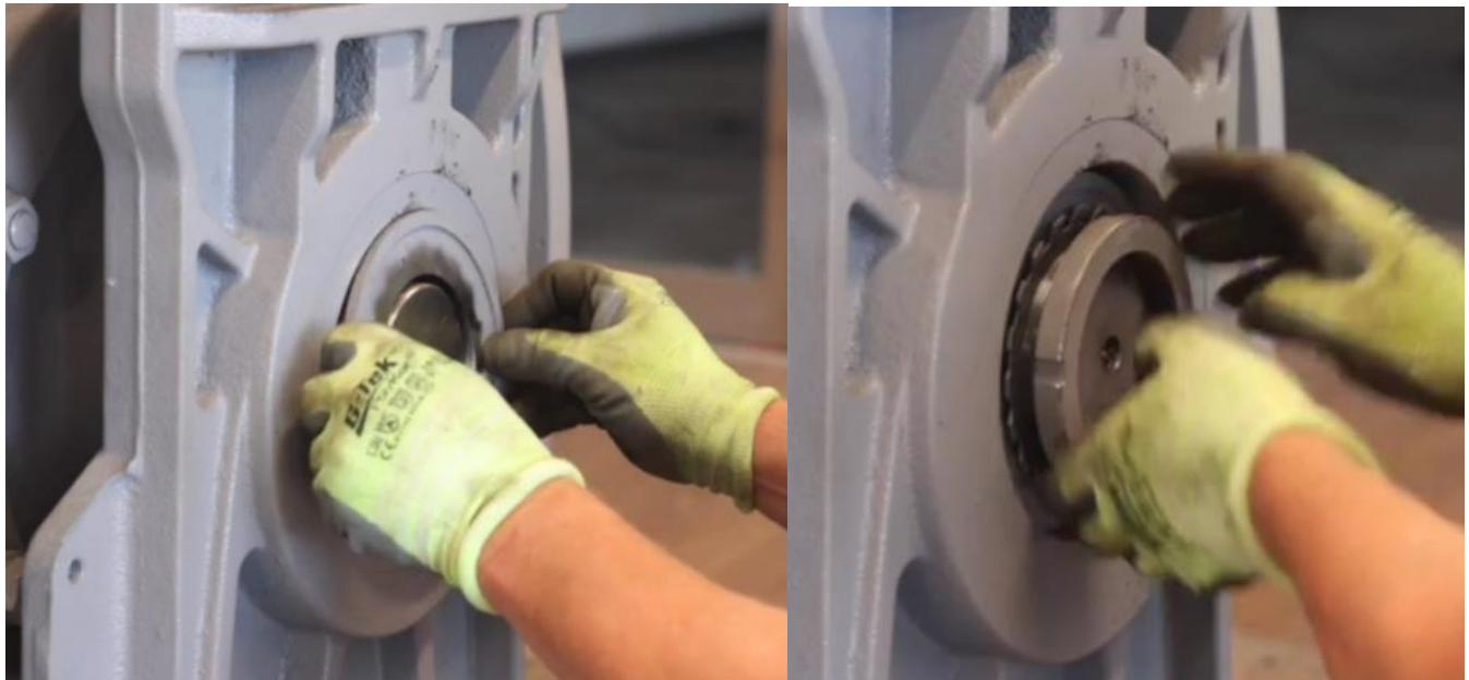
Figure 4-148: Flip Retainer Plate and Reinstall, Install Lock Washer, and Lock Nut
