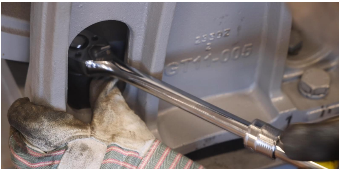
Figure 4-112: Tighten the Four Outboard Stand Bolts and Check Dial Indicator
