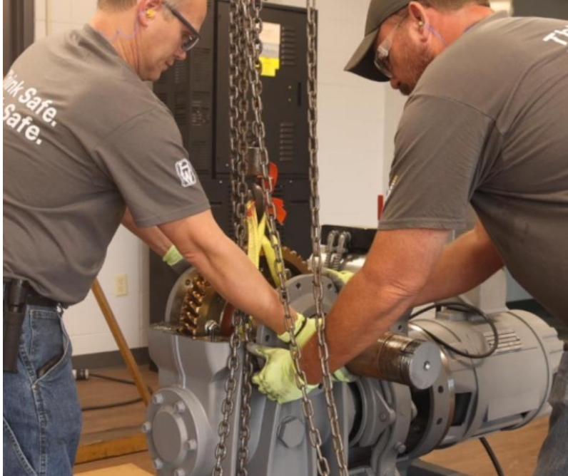
Figure 4-36: Place Hoist Straps As Shown, Remove Pressure, Remove Eccentric
