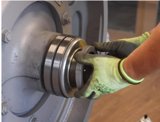
Figure 4-96: Install Shaft Lock Nut Until Snug
