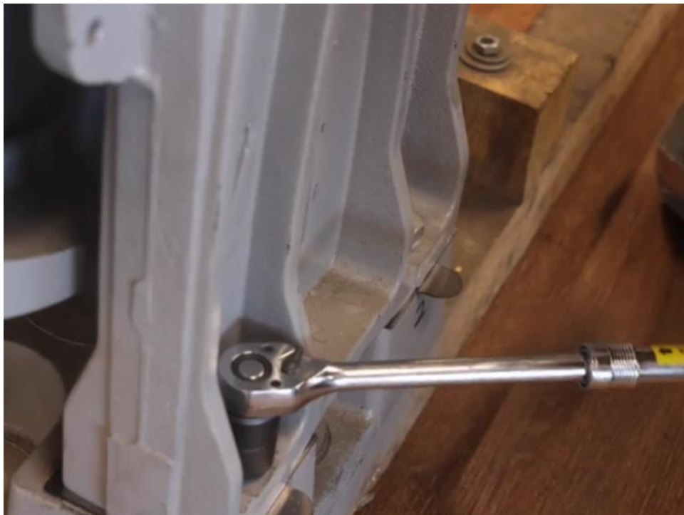
Figure 4-162: Torque Four Outboard Stand Bolts to 200 ft*lbs
