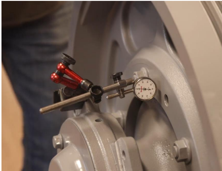
Figure 4-163: Check Backlash with Dial Indicator
