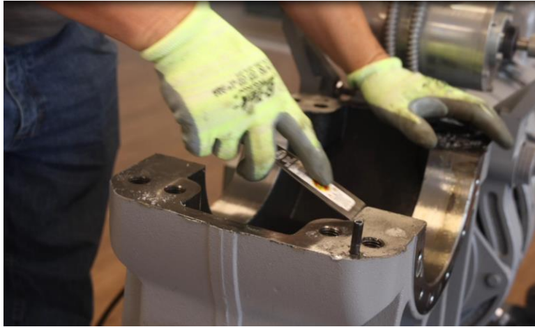
Figure 4-66: Thoroughly Clean Lower Housing
