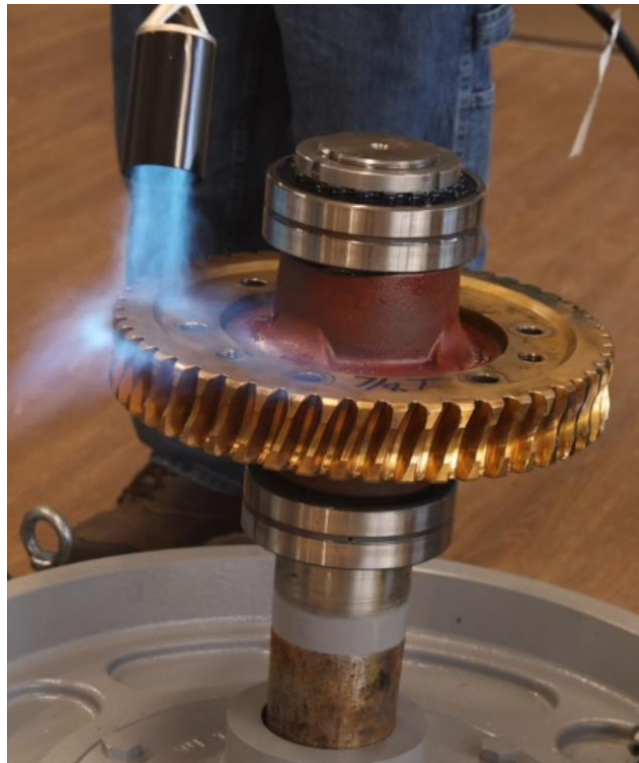
Figure 4-45: Heat Bronze Gear For Removal
