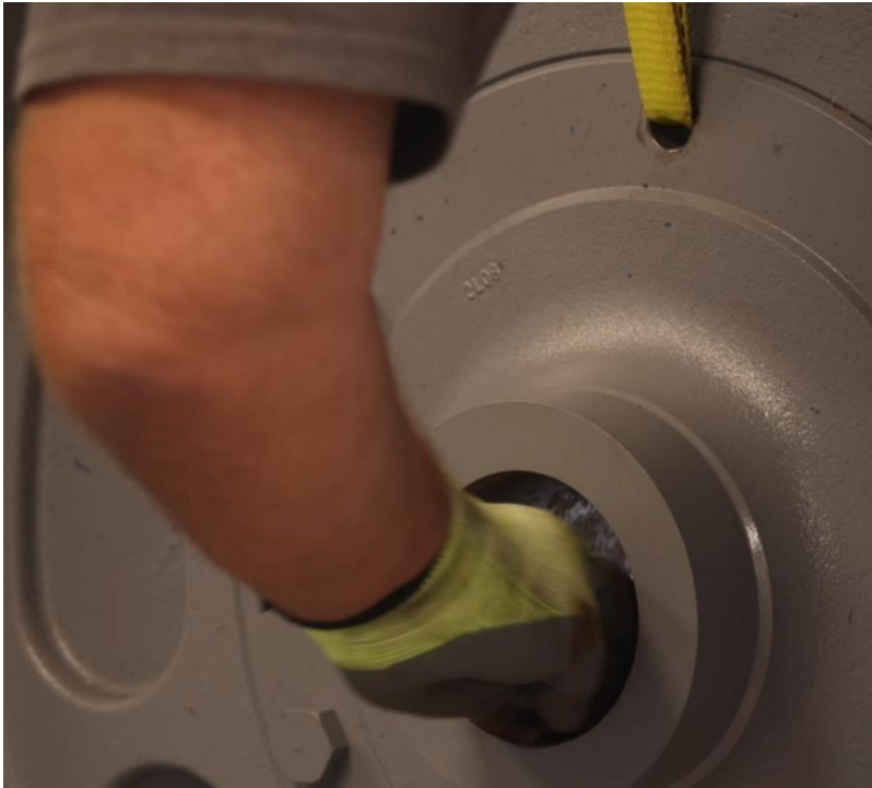
Figure 4-88: Thoroughly Clean Bore of Traction Wheel Hub
