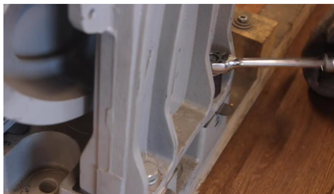
Figure 4-160: Tighten the Four Inner Outboard Stand Bolts
