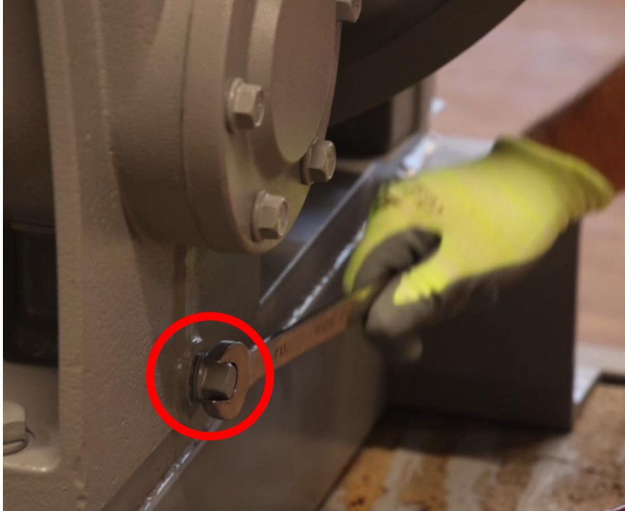
Figure 4-6: Loosen Oil Drain Plug
