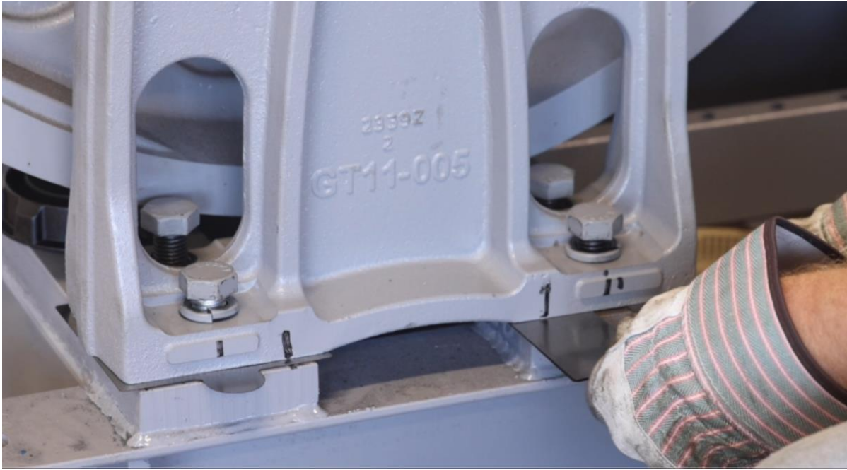
Figure 4-105: Insert Shim Packs Between Outboard Stand and Machine Base
