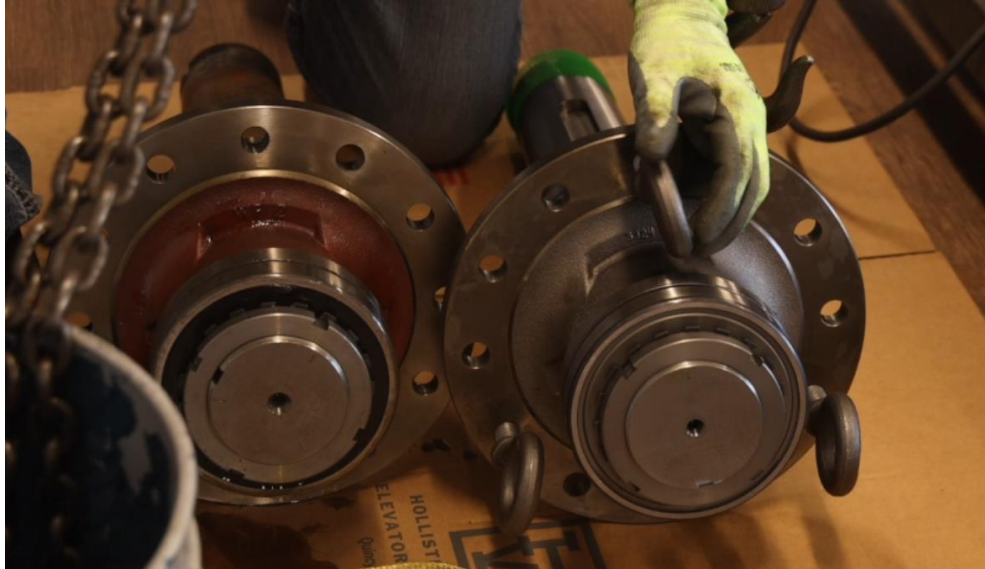
Figure 4-48: Remove Eye Bolts from Old Center Assembly and Install on New Center Assembly
