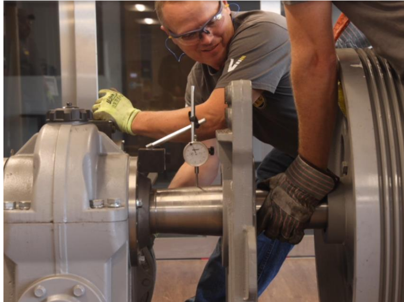
Figure 4-139: Rotate Drum By Hand While Holding the Brake Open With Manual Release Handle
