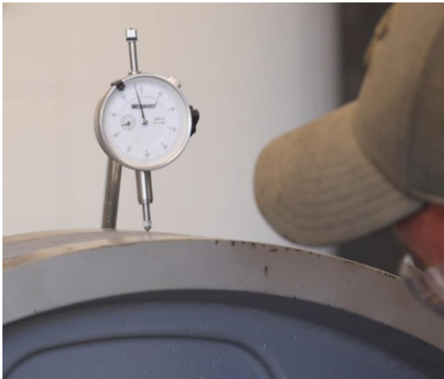
Figure 4-104: Read Dial Indicator and Record Value
