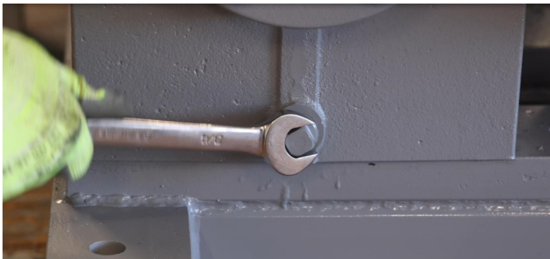
Figure 4-164: Reinstall Oil Plug and Tighten
