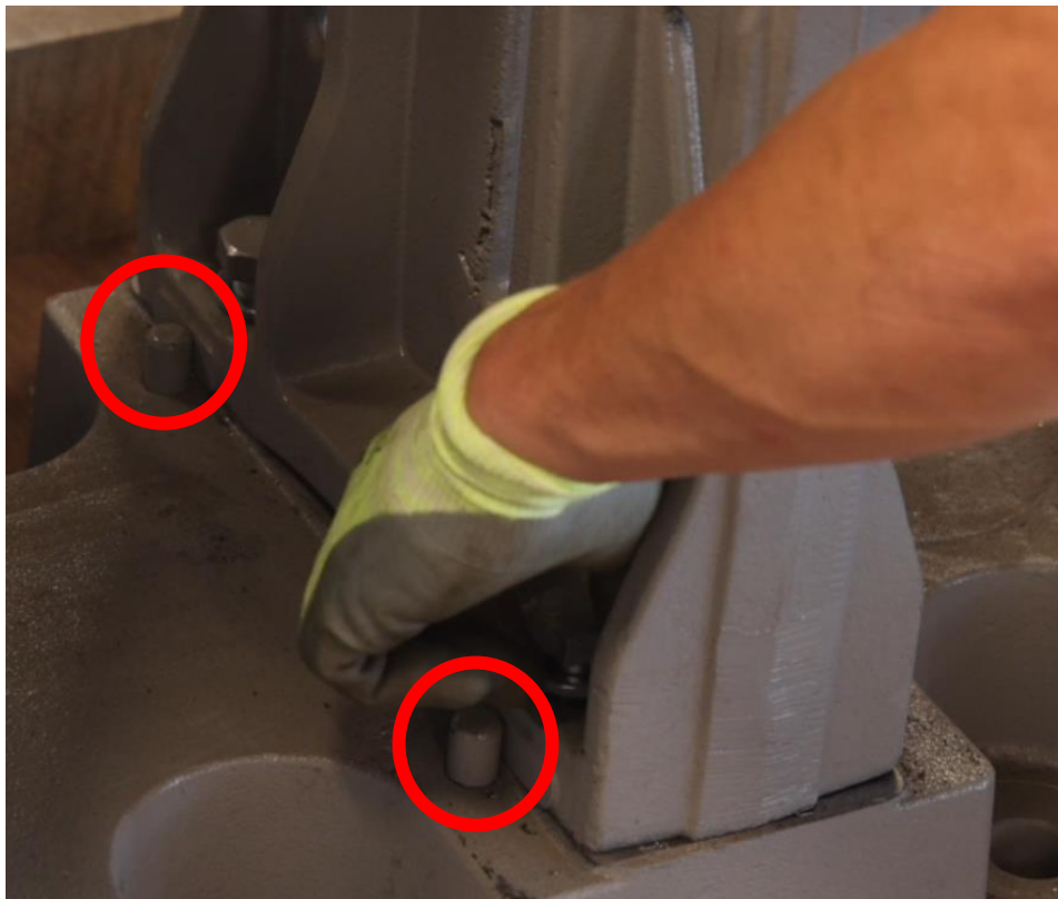
Figure 4-124: Loosely Reinstall Four Inner Outboard Stand Bolts
