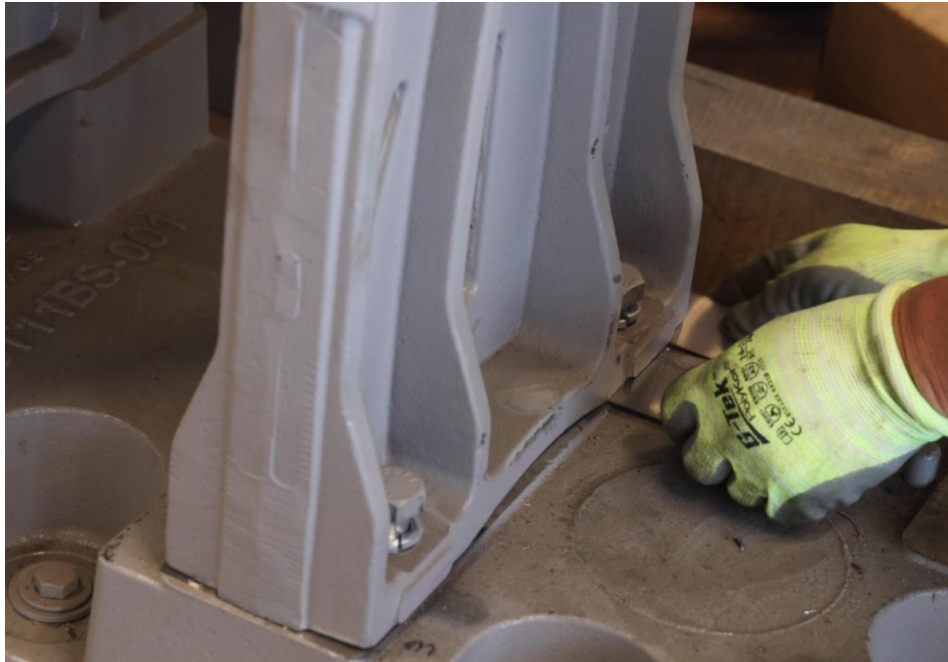
Figure 4-125: Insert Shim Packs Between Outboard Stand and Machine Base
