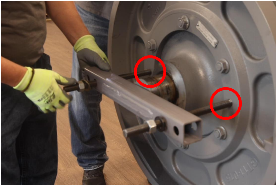
Figure 4-21: Install Traction Wheel Puller Assembly
