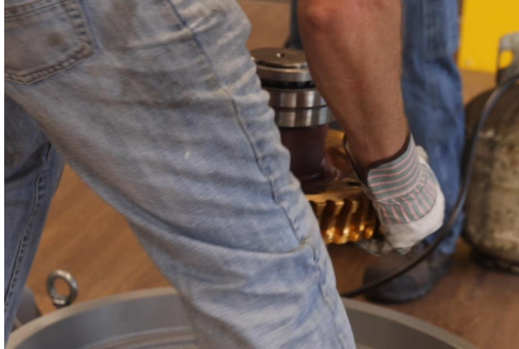
Figure 4-46: Remove Bronze Gear From Gear Hub
