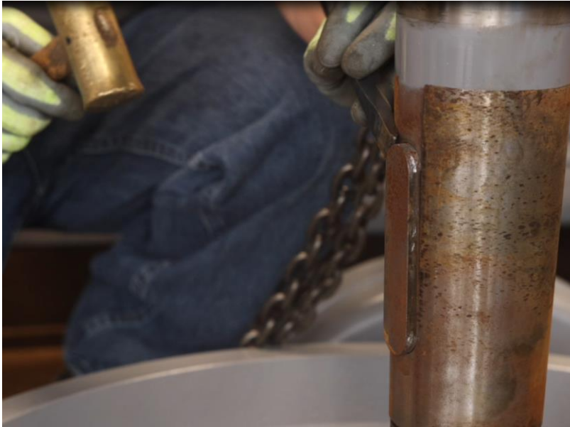
Figure 4-40: Remove Shaft Key
