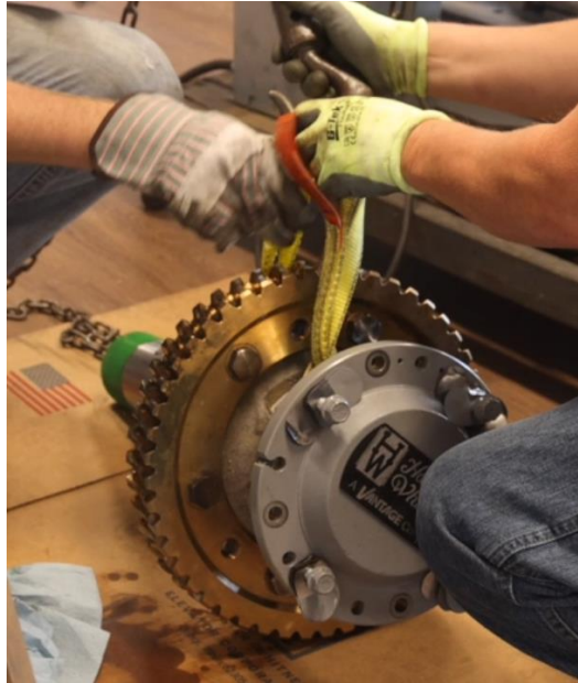
Figure 4-68: Reconfigure the Hoisting Straps
