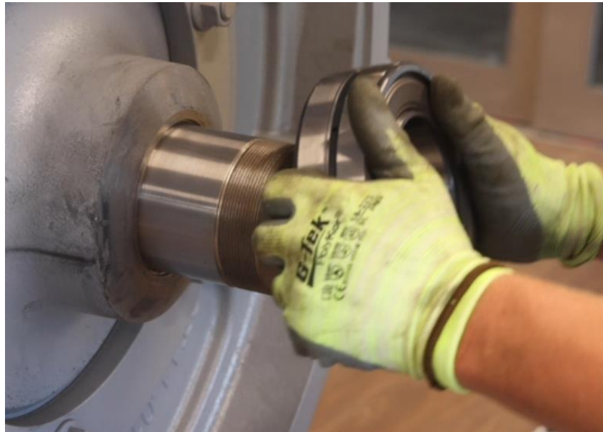
Figure 4-94: Reinstall Original Outboard Stand Bearing
