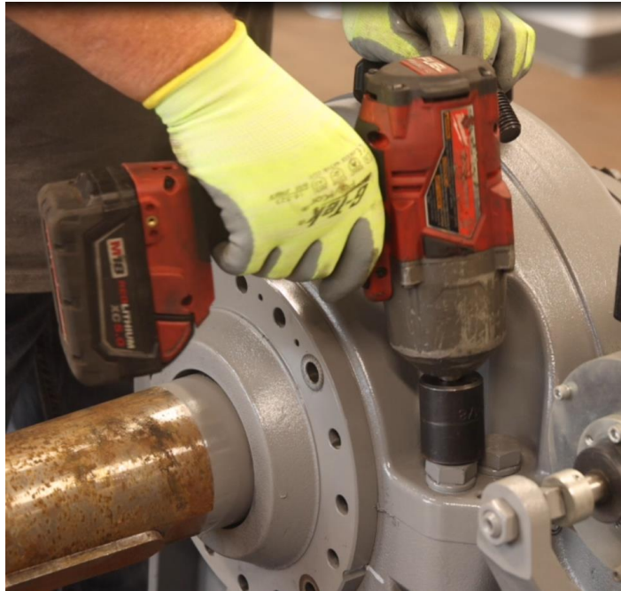
Figure 4-30: Remove the Eight Upper Housing to Lower Housing Bolts
