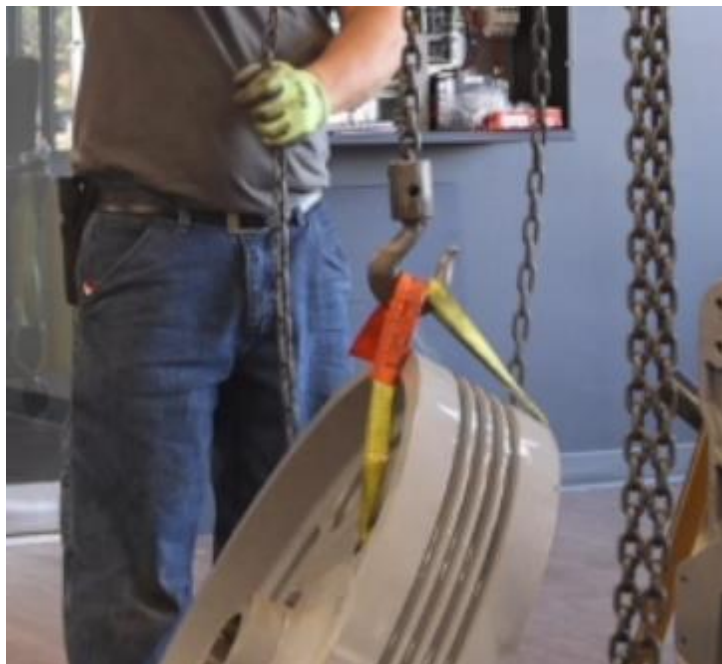
Figure 4-134: Hoist Traction Wheel Assembly To Machine
