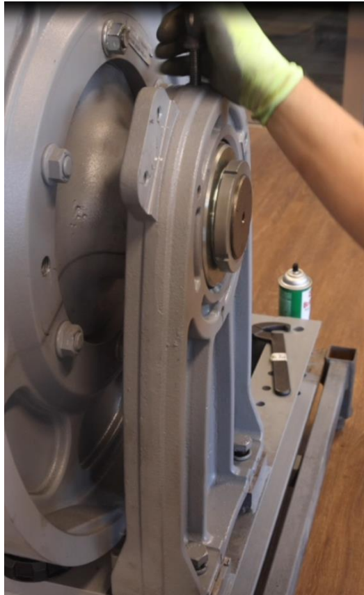
Figure 4-100: Remove Hoisting Eyebolt from Outboard Stand
