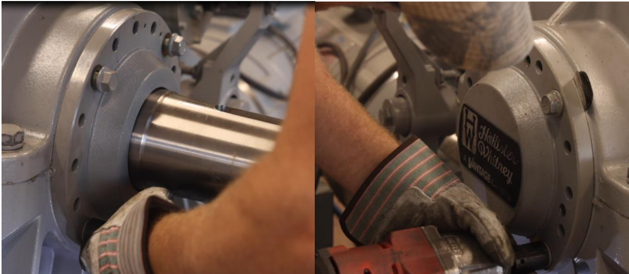
Figure 4-81: Fully Seat Both Eccentric Bolts (Quantity of 8 Bolts) – Torque to 57 ft*lbs.
