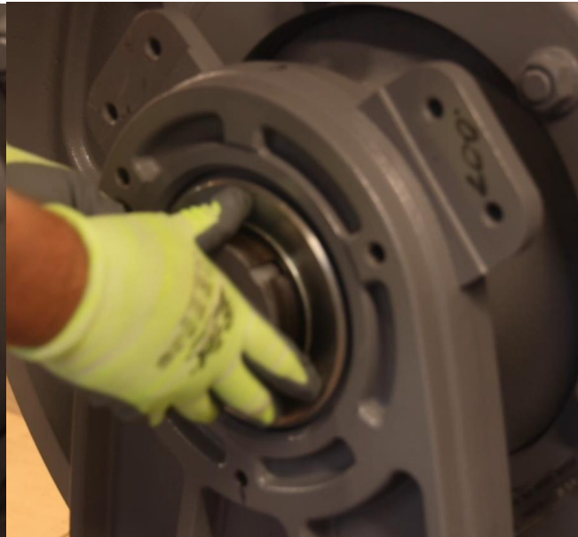
Figure 4-14: Flip and Reinstall Retainer Plate
