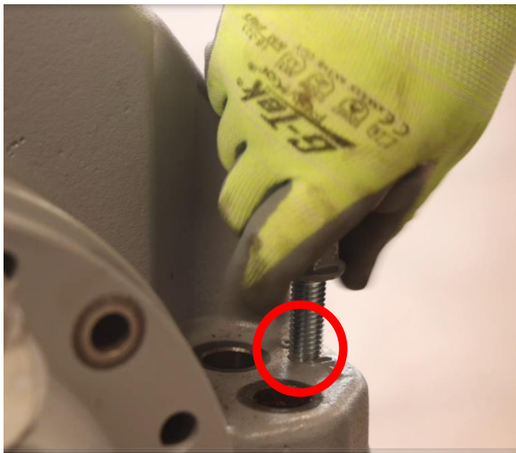
Figure 4-31: Insert Jack Bolts into Upper Housing Threaded Holes
