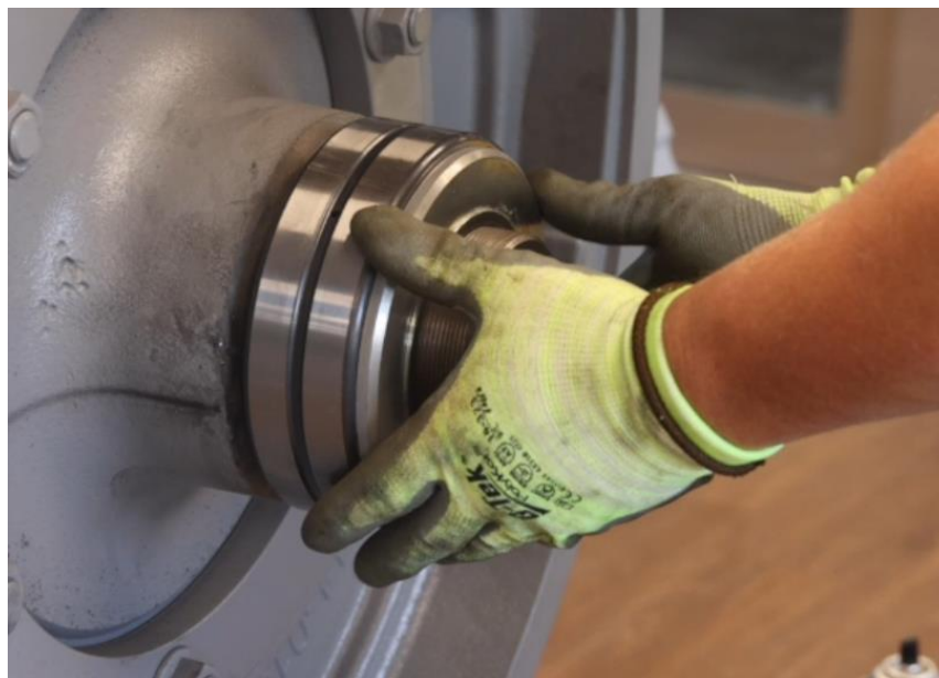
Figure 4-95: Reinstall Original Outboard Stand Bearing In This Orientation
