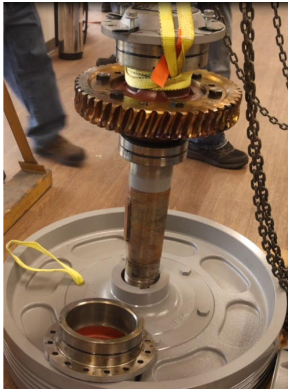
Figure 4-39: Place Center Assembly Into Traction Wheel Hub
