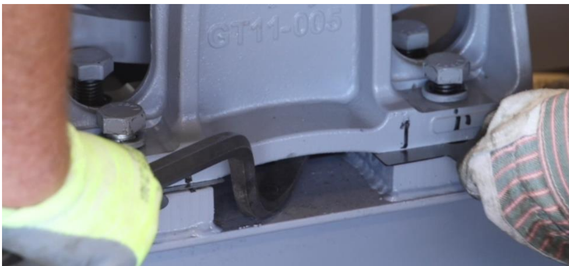
Figure 4-106: Gently Pry On Outboard Stand to Remove Shim Packs
