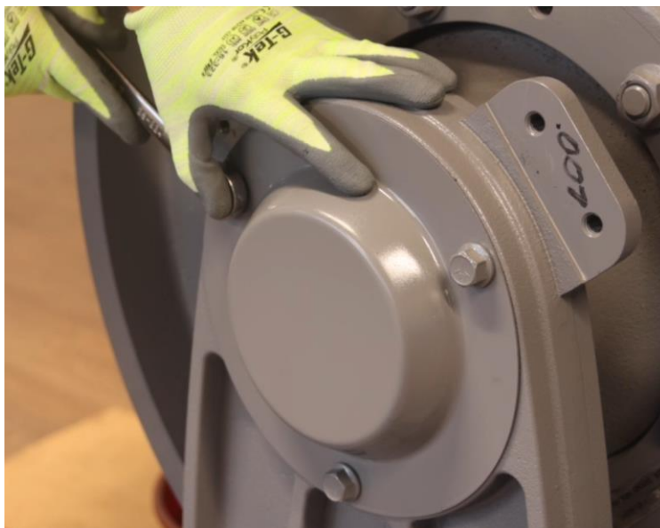
Figure 4-8: Removal of Three Cover Bolts
