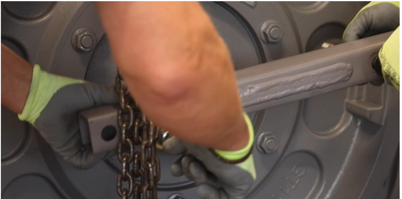
Figure 4-25: Remove Puller Assembly
