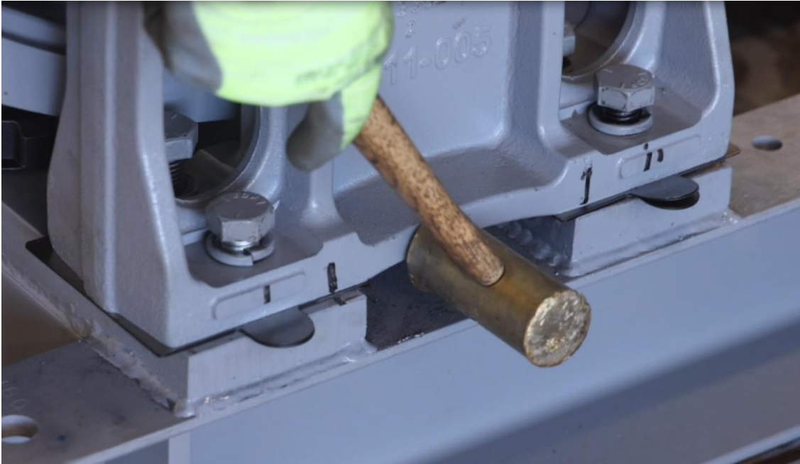
Figure 4-111: Gently Tap Bottom of Outboard Stand to Align Dowel Pins to Outboard Stand
