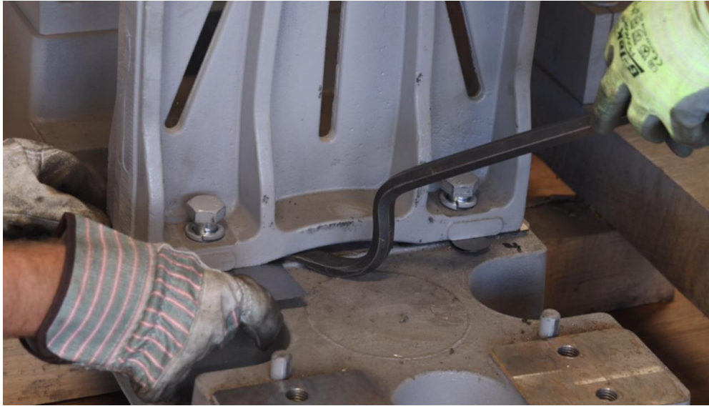
Figure 4-127: Pry Outboard Stand Up to Insert Thicker Shim Packs
