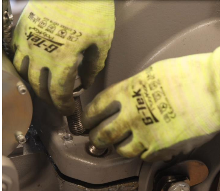
Figure 4-77: Partially Reinstall Upper Housing to Lower Housing Bolts – Do Not Tighten
