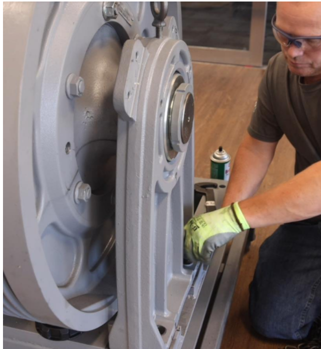
Figure 4-99: Loosely Install the Four Outboard Stand Mounting Bolts
