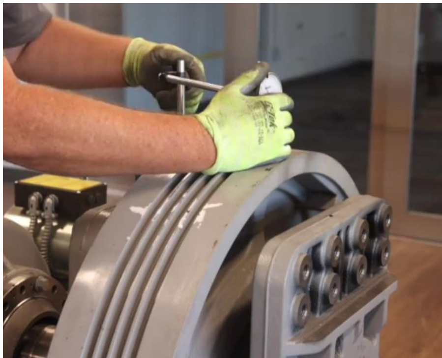
Figure 4-152: Place Dial Indicator on Traction Wheel
