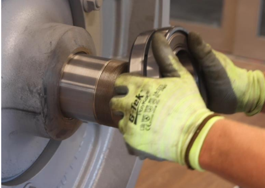
Figure 4-141: Reinstall Original Outboard Stand Bearing
