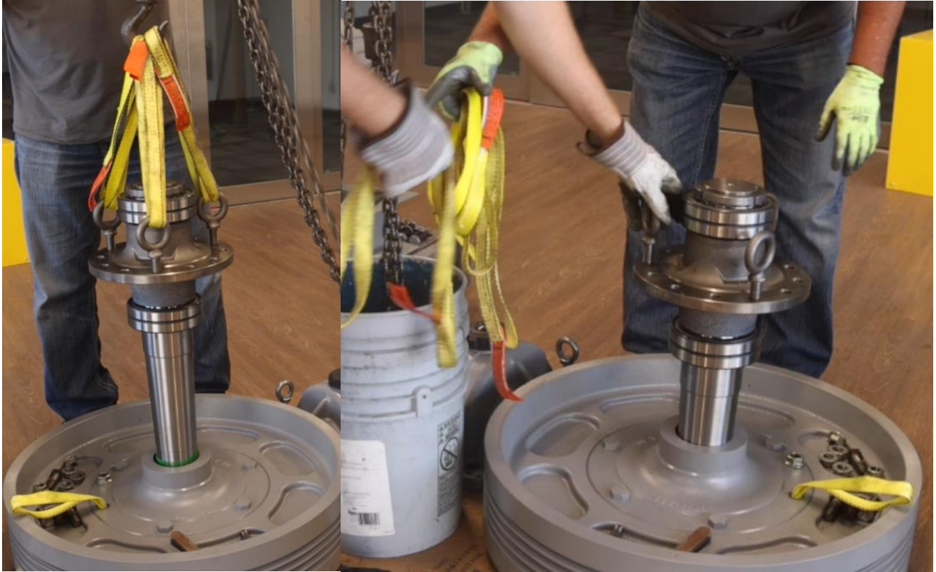
Figure 4-50: Place New Center Assembly into Traction Wheel
