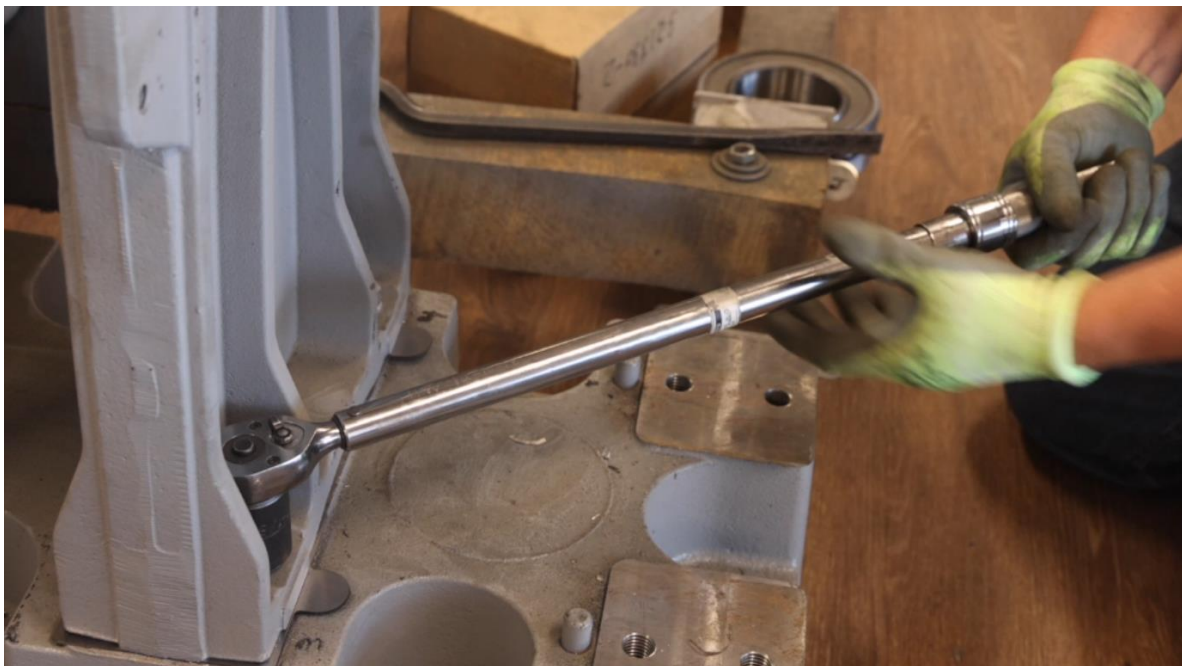
Figure 4-132: Torque Four Outboard Stand Bolts to 200 ft*lbs
