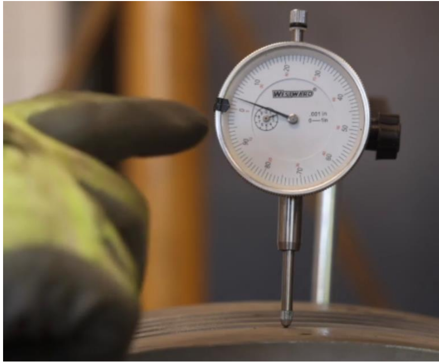
Figure 4-161: After Tightening Bolts Ensure Dial Indicator Still Reads Above Zero
