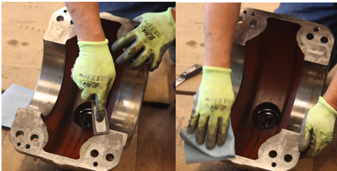
Figure 4-72: Thoroughly Clean Upper Housing
