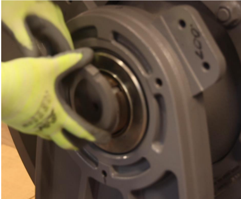
Figure 4-15: Reinstall Lock Nut
