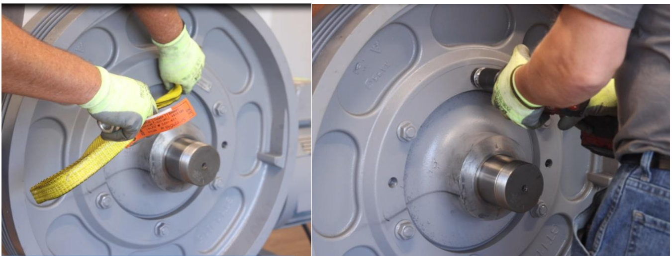
Figure 4-93: Remove Strap and Reinstall Original Wheel Body Bolt
