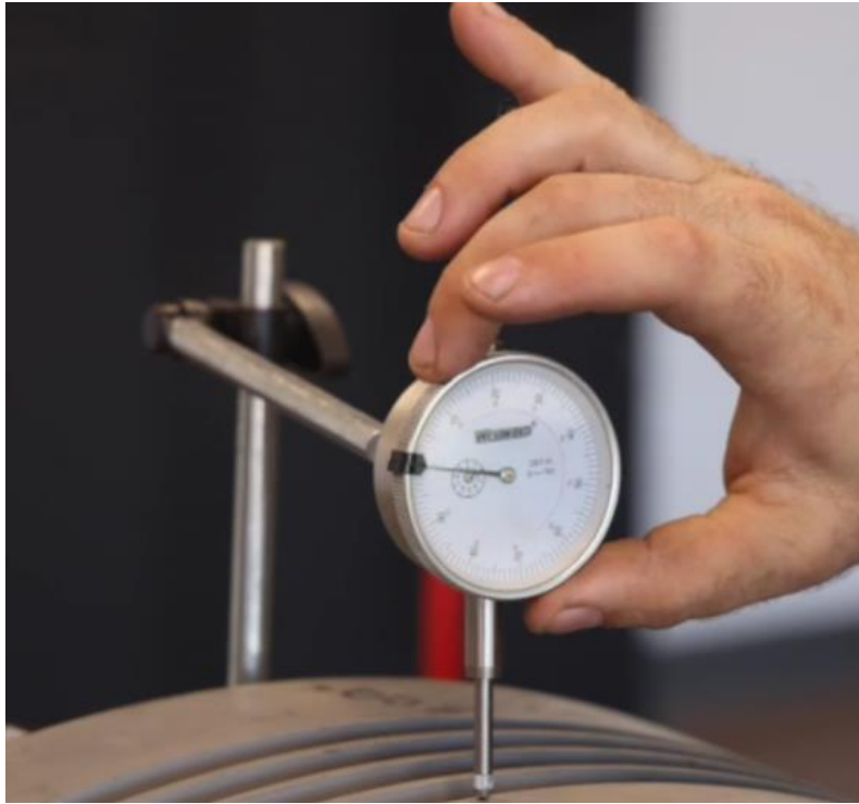
Figure 4-153: Zero Dial Indicator
