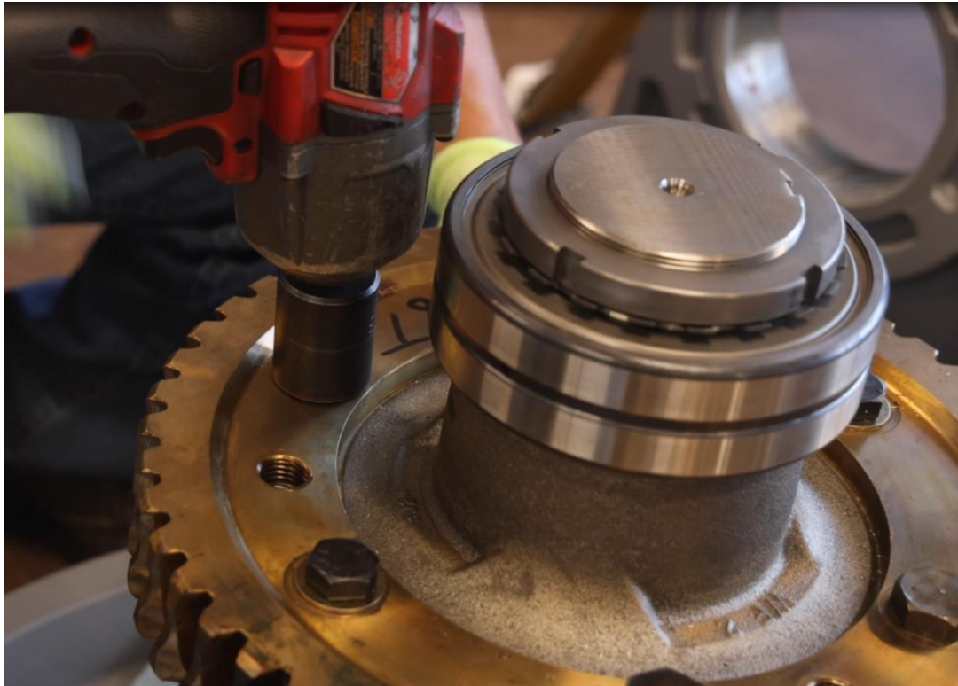
Figure 4-58: Install Four of the Original Nuts and Bolts – Torque to 200 ft*lbs.
