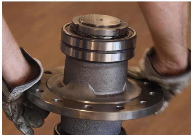
Figure 4-51: Clean and Deburr Gear Hub
