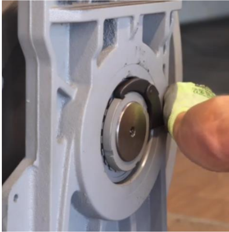
Figure 4-149: Fully Tighten Shaft Lock Nut
