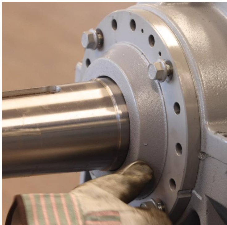
Figure 4-78: Partially Thread Traction Wheel Side Bolts
