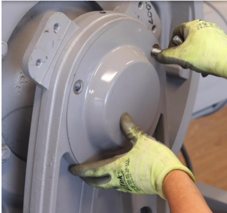
Figure 4-119: Reinstall Bearing Cover and Bearing Cover Bolts
