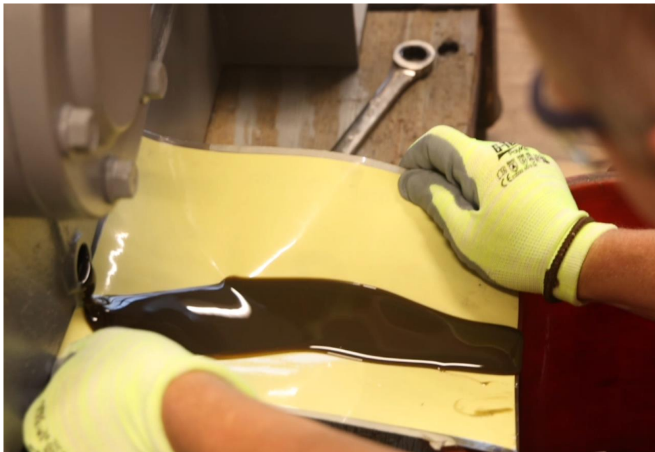
Figure 4-7: Drain Oil into Clean Bucket
