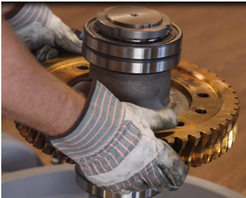
Figure 4-55: Rotate Gear to Align Unthreaded Holes
