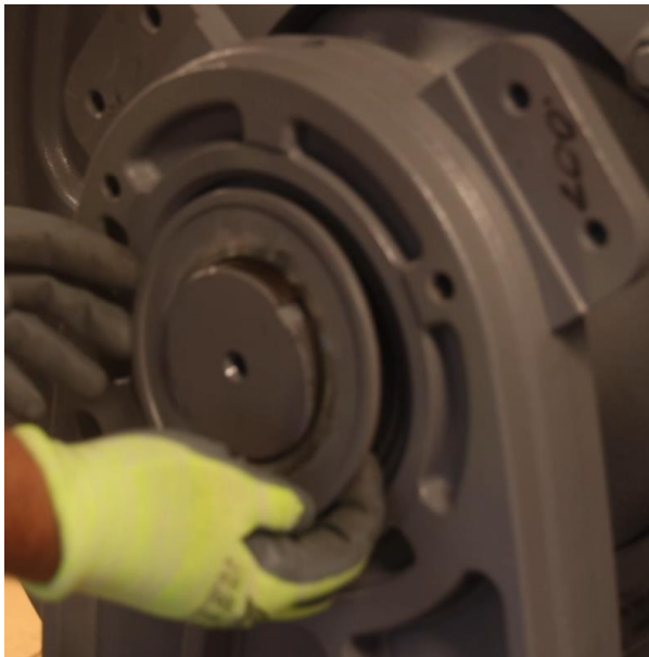
Figure 4-13: Remove Retainer Plate
