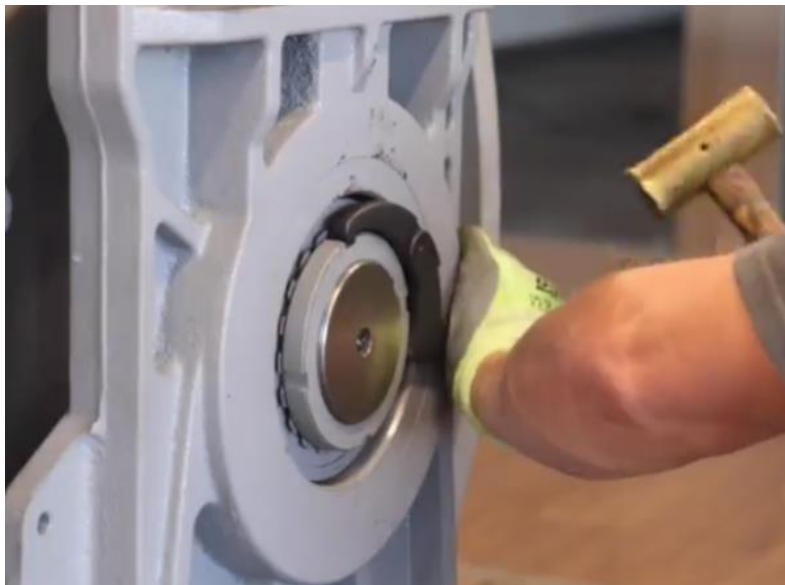
Figure 4-150: Hit with Brass Hammer to Ensure Lock Nut is Tight
