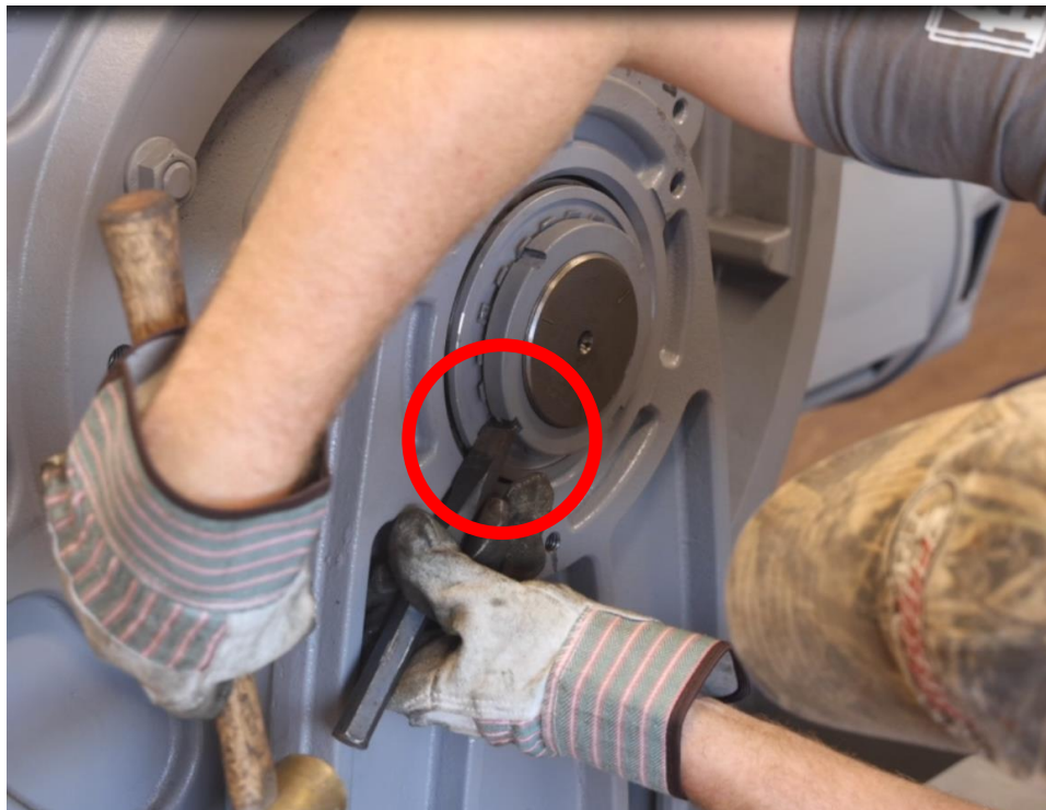
Figure 4-118: Bend Washer Lock Tab into Slot in Lock Nut
