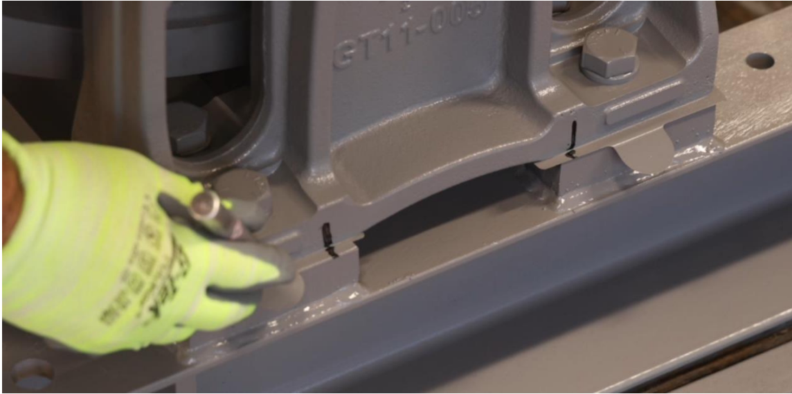
Figure 4-4: Mark Position of Shim Packs
