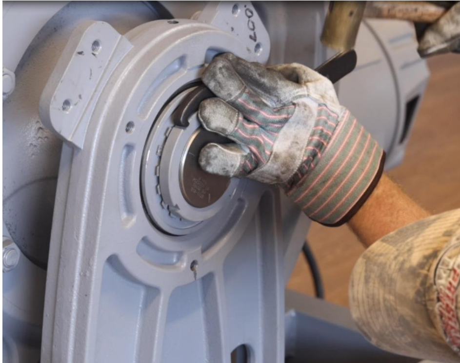
Figure 4-117: Hit with Brass Hammer to Ensure Lock Nut is Tight
