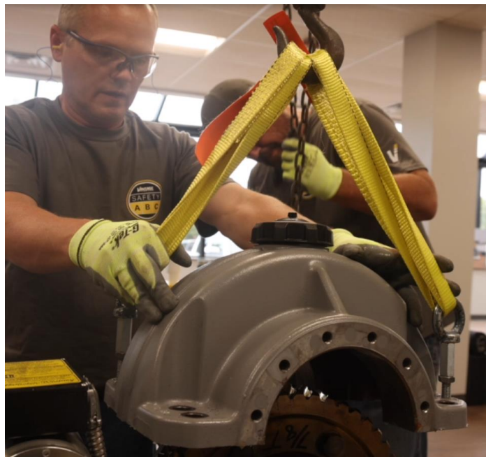
Figure 4-35: Install Eyebolts and Hoist Upper Housing from Lower Housing
