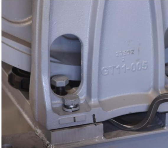
Figure 4-103: Pry Up on the Outboard Stand
