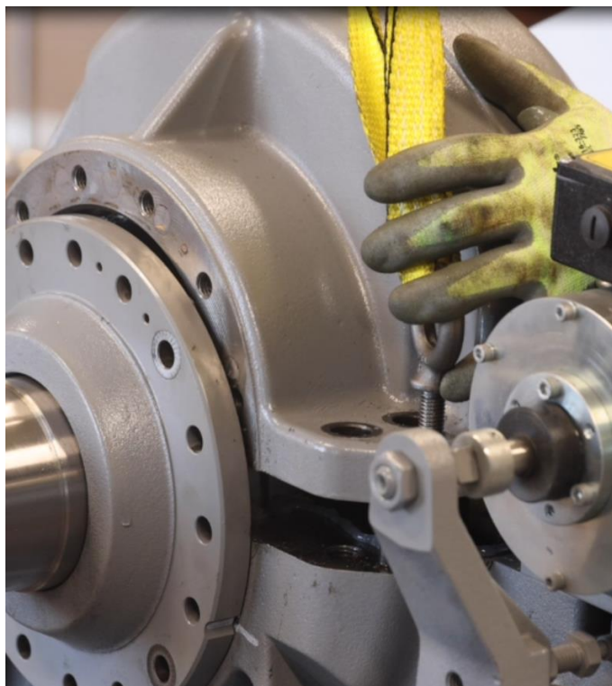
Figure 4-76: Lower Upper Housing Onto Lower Housing
