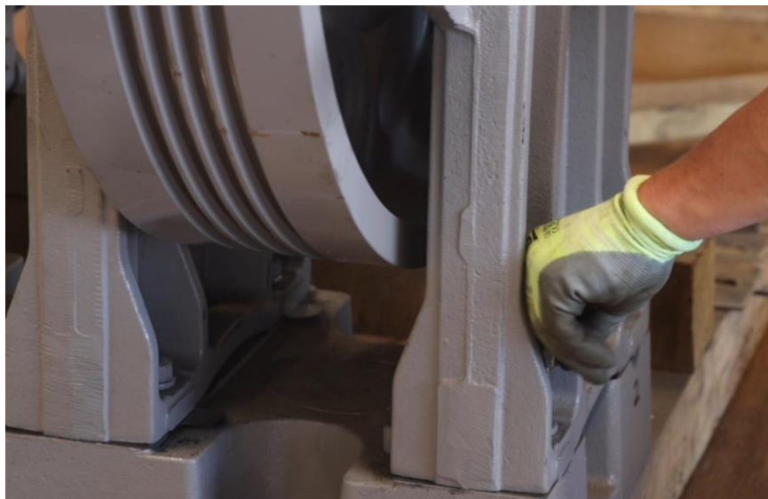
Figure 4-146: Loosely Reinstall Four Outer Outboard Stand Bolts
