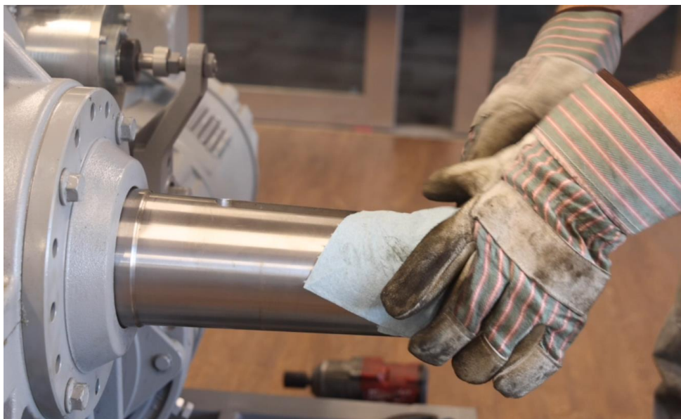
Figure 4-87: Thoroughly Clean End of Shaft
