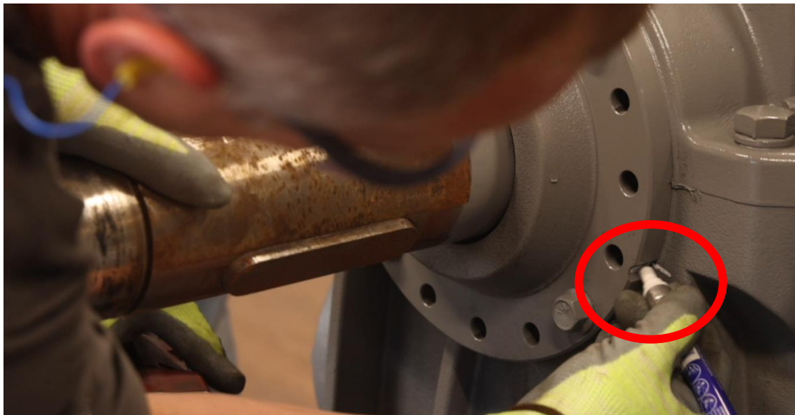
Figure 4-27: Mark Position of Eccentric Notch Relative to Lower Housing
