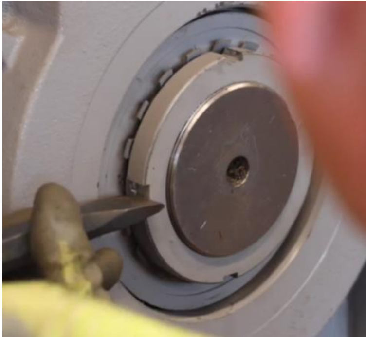
Figure 4-151: Bend Washer Lock Tab into Slot in Lock Nut
