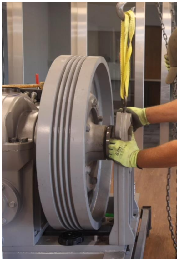
Figure 4-97: Install Outboard Stand Over Bearing
