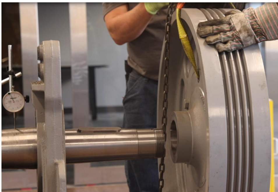
Figure 4-138: Hoist Traction Wheel Assembly and Align To Shaft
