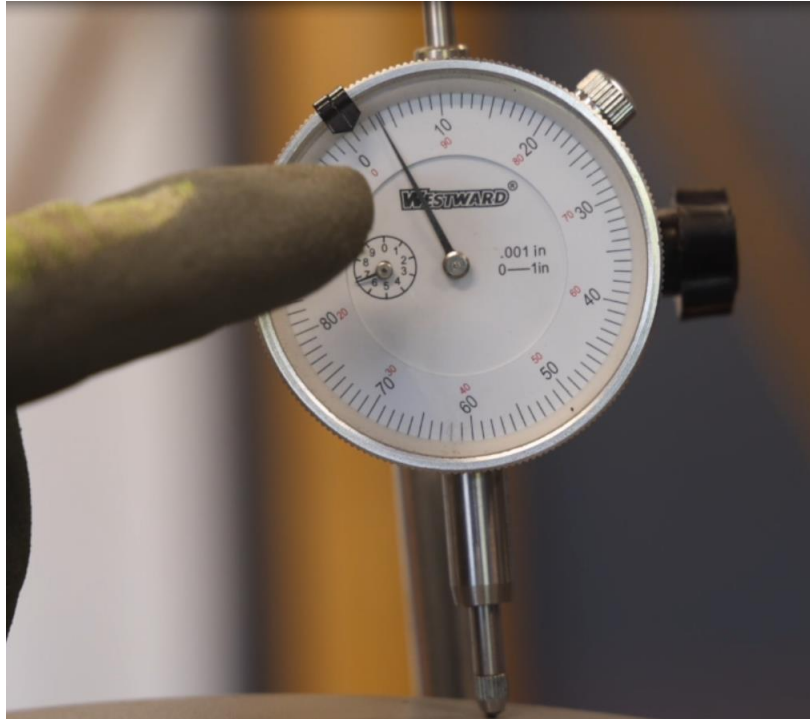
Figure 4-109: Add Enough Shims to Get Appropriate Dial Indicator Reading
