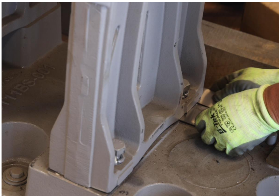
Figure 4-156: Insert Shim Packs Between Outboard Stand and Machine Base
