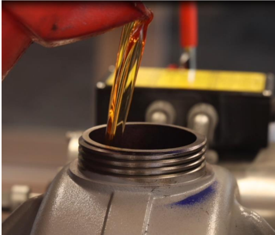
Figure 4-165: Fill Gearbox with Original Oil
