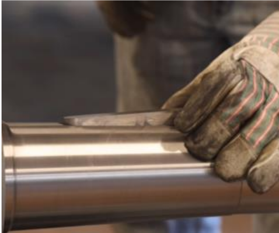
Figure 4-135: Reinstall Original Shaft Key
