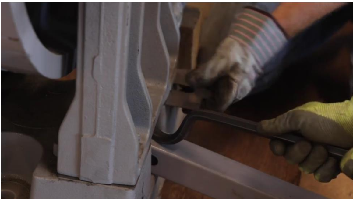
Figure 4-158: Pry Outer Outboard Stand Up to Insert Thicker Shim Packs
