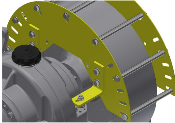
Figure 4-9: GT11 Bracket Mounting Illustration
