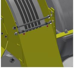
• Loosely (Whiz Bolts finger tight) attach the Bottom Extension Angles to the Lower Cover and slip the Lower Cover into place within the Upper Cover.
