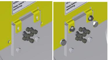
• For 63 and 74 Series Machines, set the Outboard Side Plate Bracket in place. Make sure the top edge of the bracket is horizontal with the machine and securely bolt in place.
