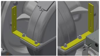
• Attach the Inboard Side Plate Bracket to the Housing Brackets as shown. Bolts should be finger tight for later positioning.
