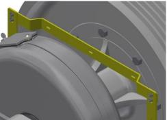
• If included, attach supplemental Side plate Bracket to each Housing Bracket.
