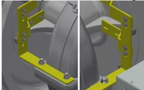
• Attach the Side Plate Bracket as shown and snug the bolts down.
