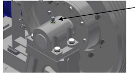
• Slip the Side Plate Bracket under the washer and position the bracket as shown. Snug down the Jam Nut finger tight.
