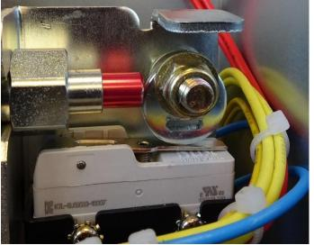
3. Using the ½" Socket or Nut Driver, turn (if necessary) the Locking Nut so that the top and bottom flats are horizontal, or parallel with the tab.
