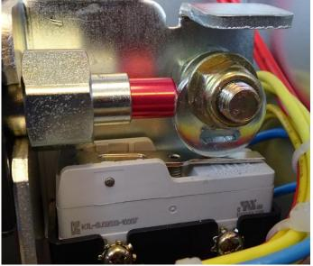
2. Using the Flat Blade Screwdriver, turn the Actuation Cam clockwise so that the Auto/Manual Microswitch is activated.
