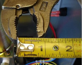
4. With the Locking Pliers handles closed (locked), adjust the open Jaws using the tab as a guide. This should be between 13/16" and 3/4" (0.8125-0.75") wide.
