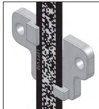
Figure 2-7: Guide Clip without Door Zone Bridge
