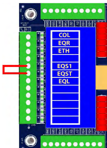
Figure 3-3: Earthquake I/O Expansion Board (if used)
