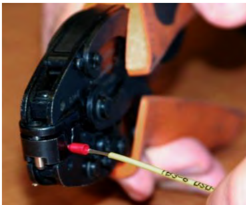
Figure 0-1 Crimp Tool for Ferrule
