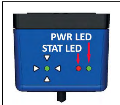
Figure 2-16: LED Array on APS Camera
