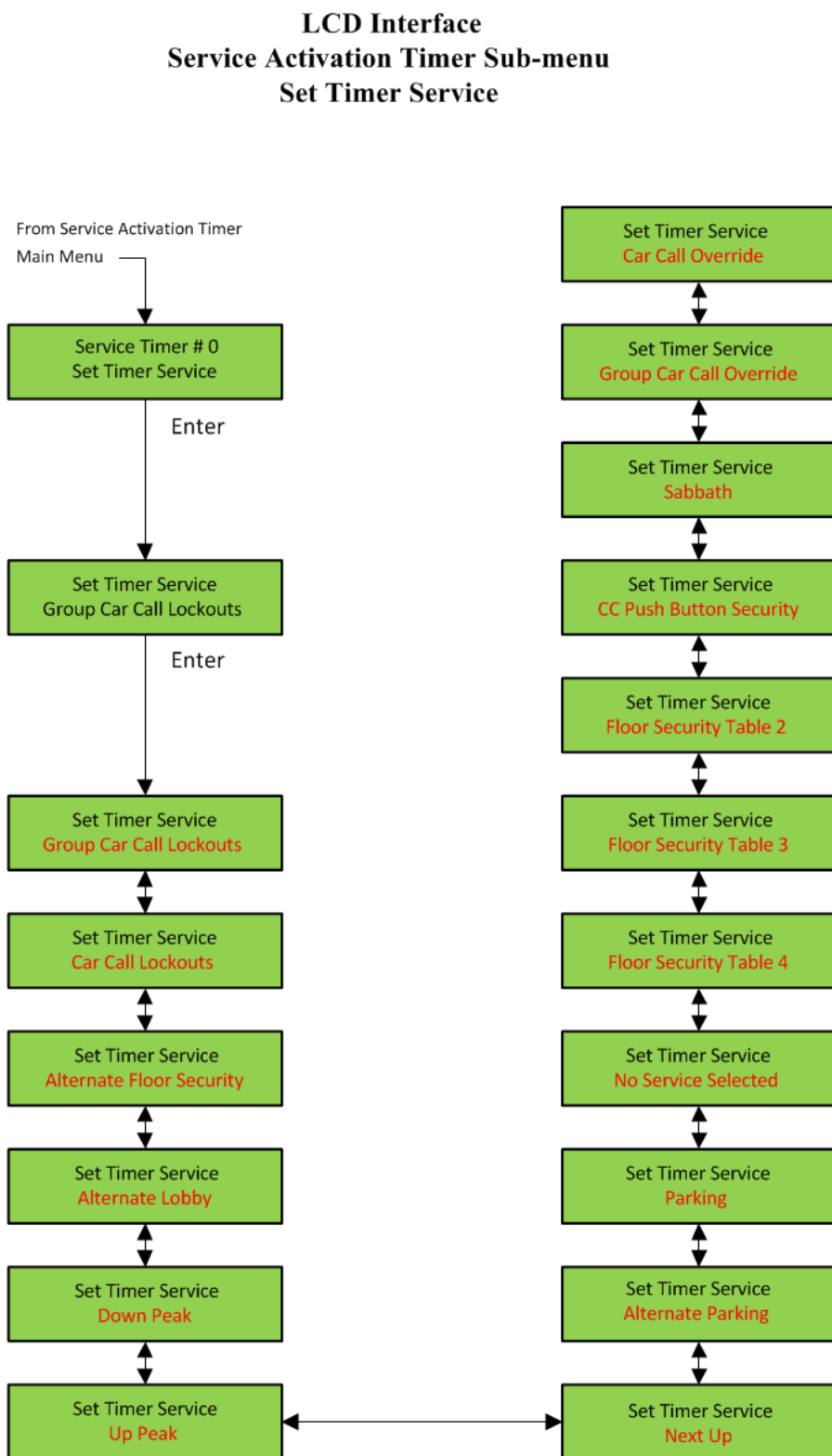
Figure 5-36: Service Activation Timer Submenu – Set Timer Service
