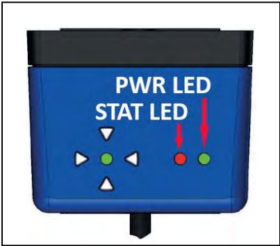
Figure 2-16: LED Array on APS Camera
