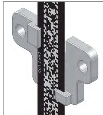
Figure 2-7: Guide Clip without Door Zone Bridge
