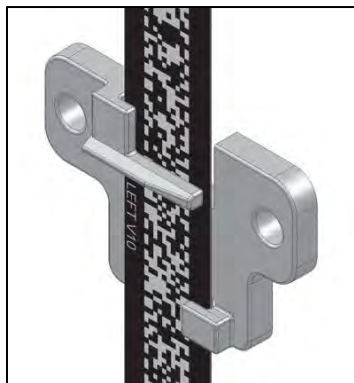
Figure 2-6: Guide Clip with Door Zone Bridge
