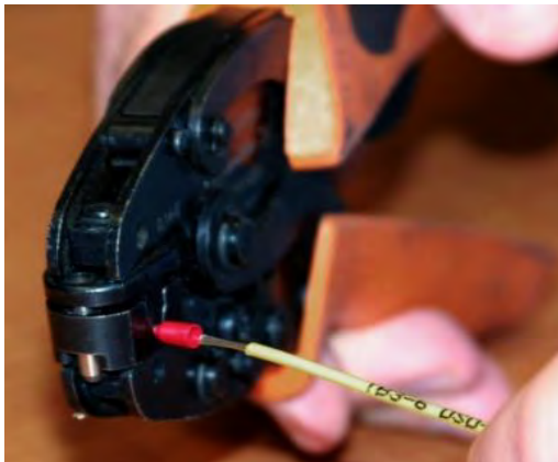
Figure 0-1 Crimp Tool for Ferrule
